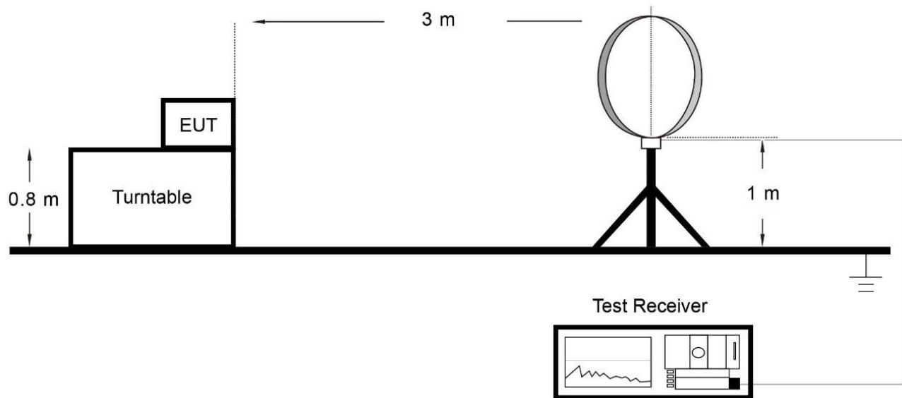
Below 1GHz Test Setup:
