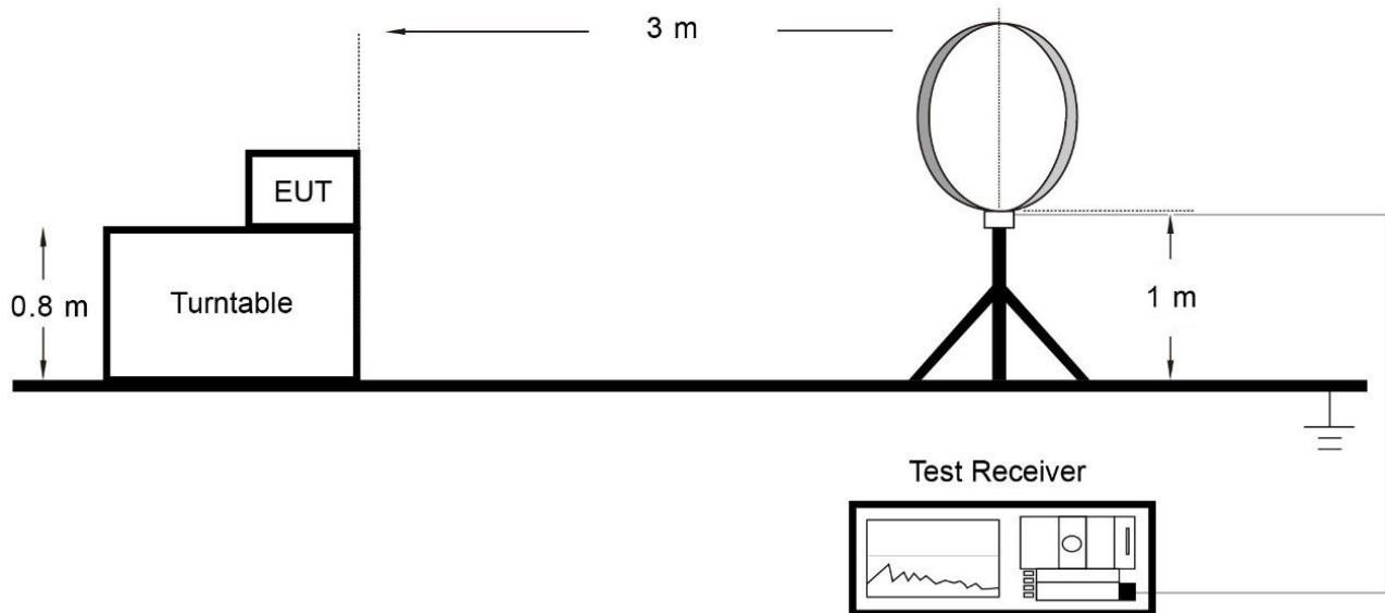
Below 1GHz Test Setup:
