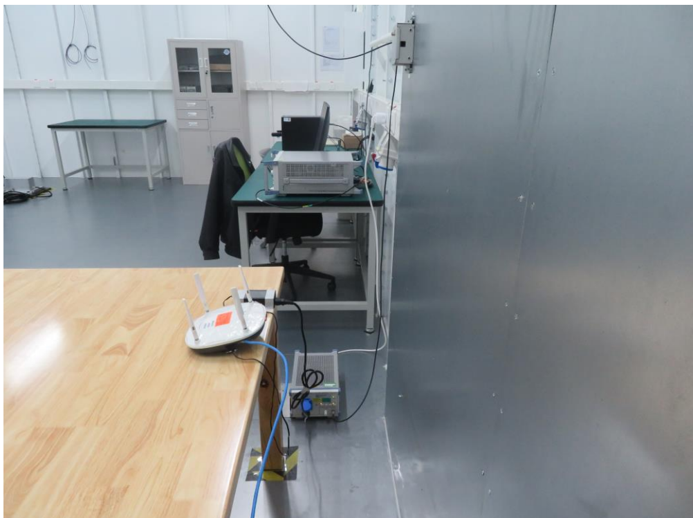
Description: Back View of Conducted Emission Test Setup for Power Port for APIN0514
