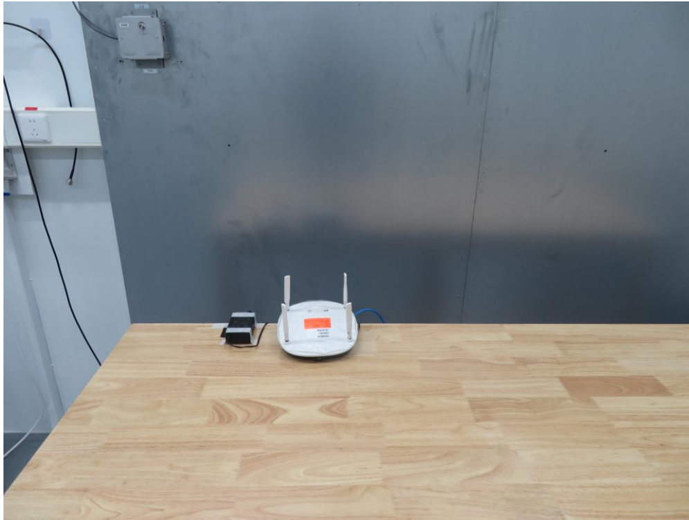
Description: Back View of Conducted Emission Test Setup for Power Port for APIN0514
