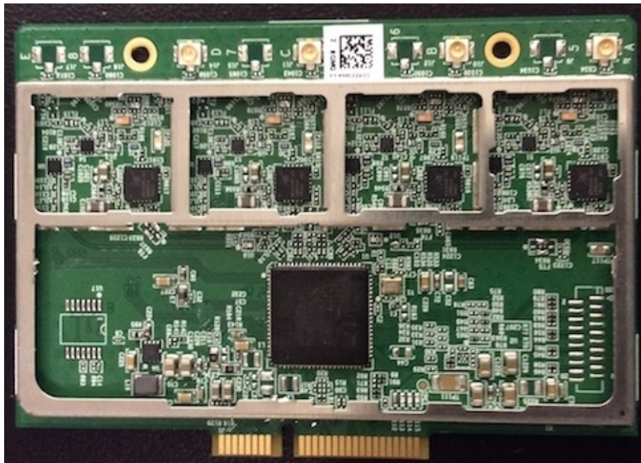
AP-325 5GHz Card (Top - Shield Removed)
