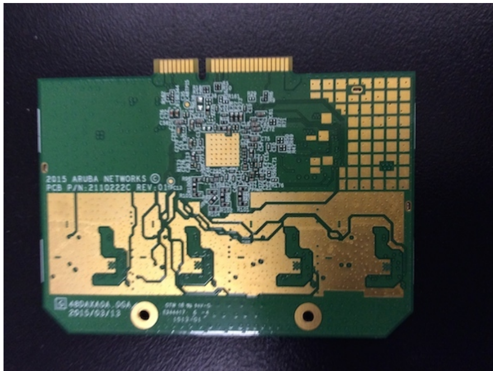
2.4GHz Card (Bottom – Plate Removed) Note: Same card used in the AP-324 & AP-325
