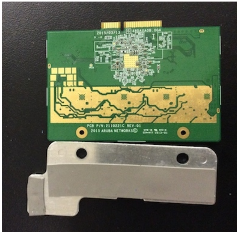
AP-325 5GHz Card (Bottom - Plate Removed)
