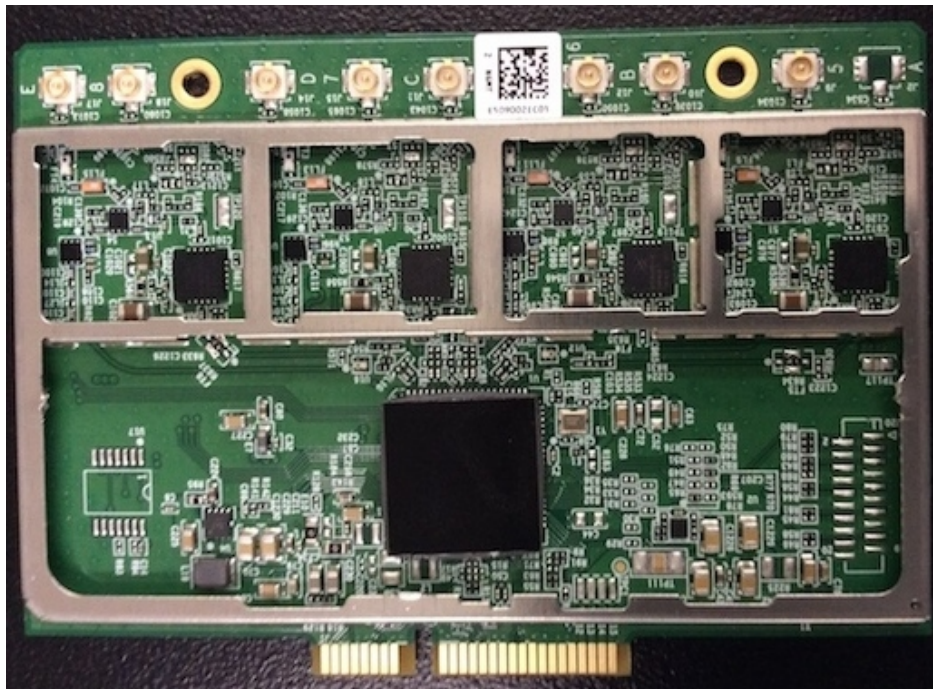
AP-324 5GHz Card (Shield Removed)
