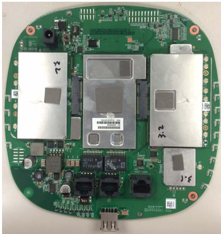
Bottom View of the Main Board PCB with Shield
