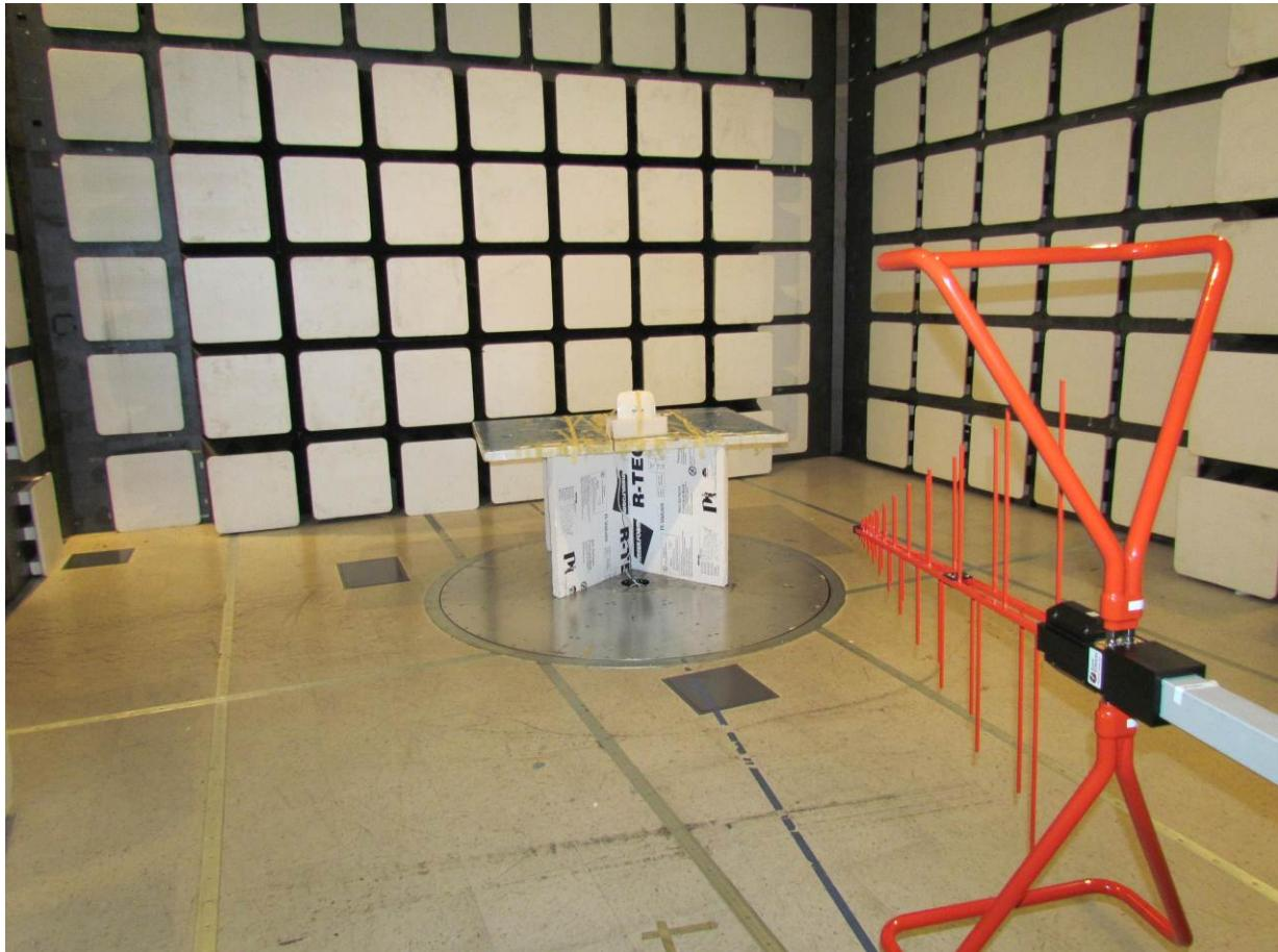
Radiated Emissions Test Setup >1 GHz
