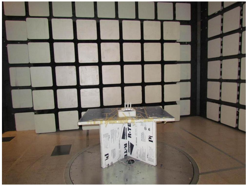
ac Wireline Test Setup >1 GHz
