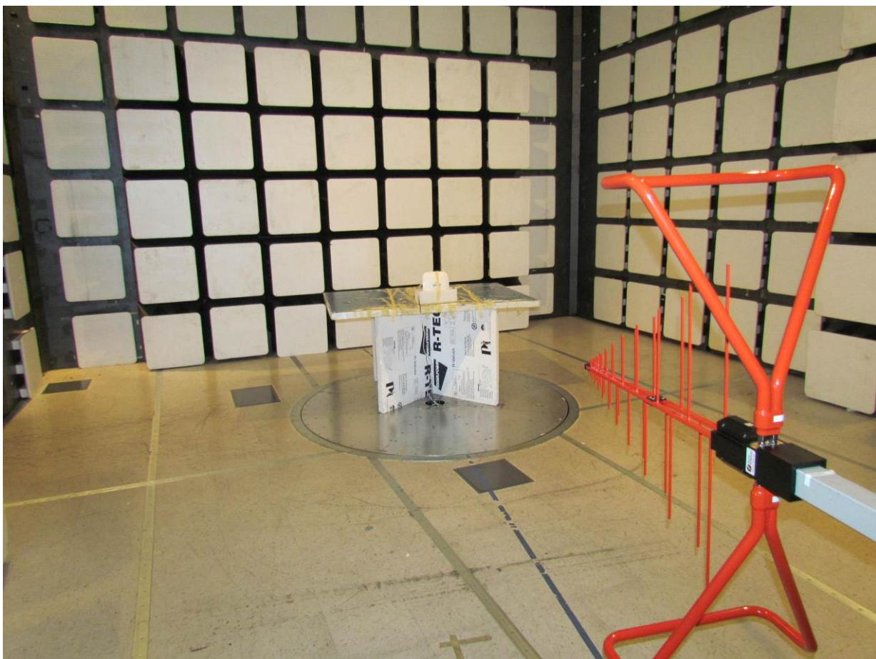
Radiated Emissions Test Setup >1 GHz
