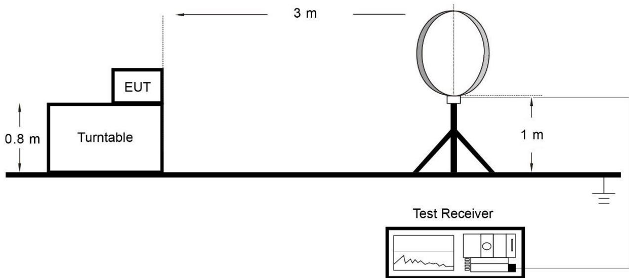
Below 1GHz Test Setup:
