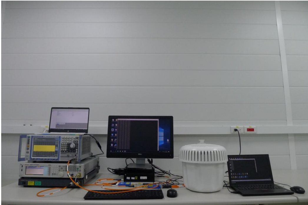
Description: DFS Radiated Test Setup
