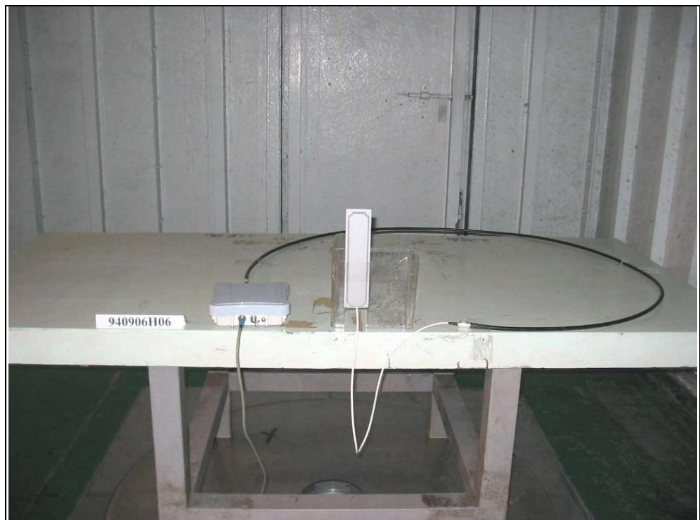
RADIATED EMISSION TEST (Antenna: AP-ANT-89)
