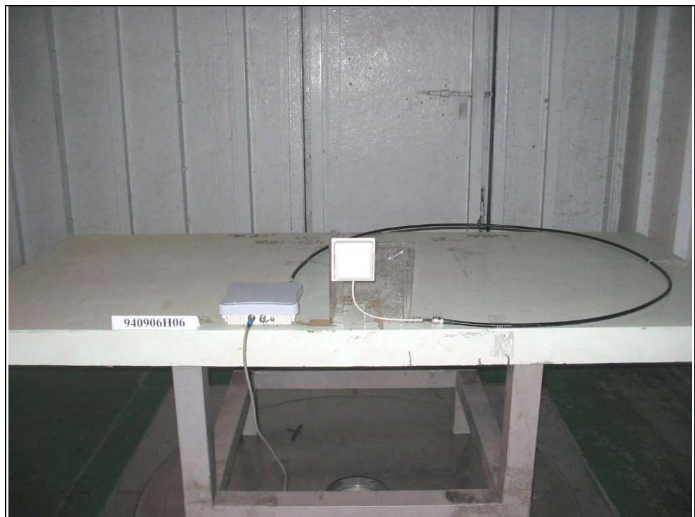
RADIATED EMISSION TEST (Antenna: AP-ANT-88)
