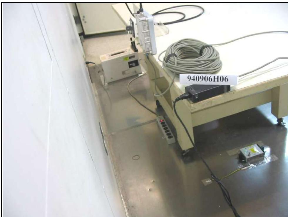
RADIATED EMISSION TEST (Antenna: AP-ANT-86)
