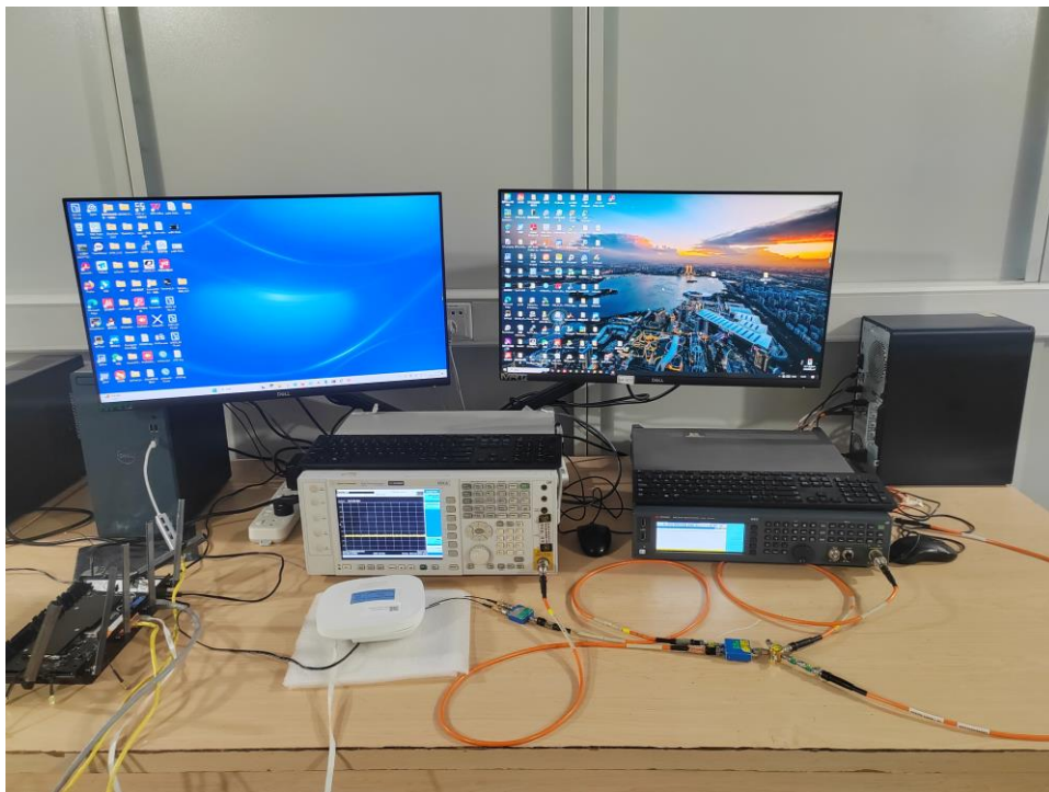
Description: Dynamic Frequency Selection Test Setup
