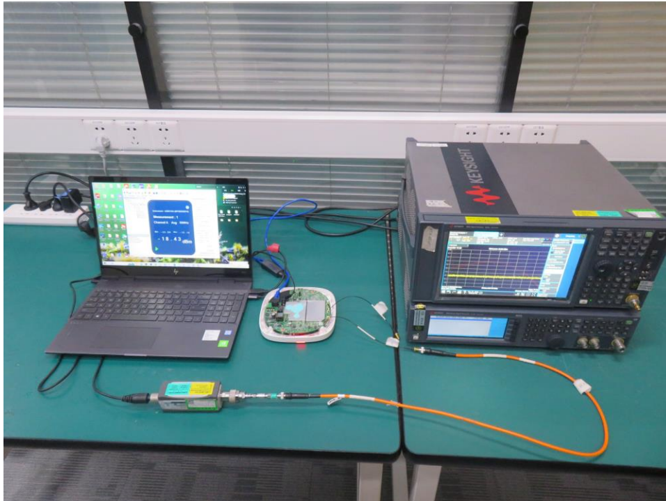
Description: Conducted Test Setup
