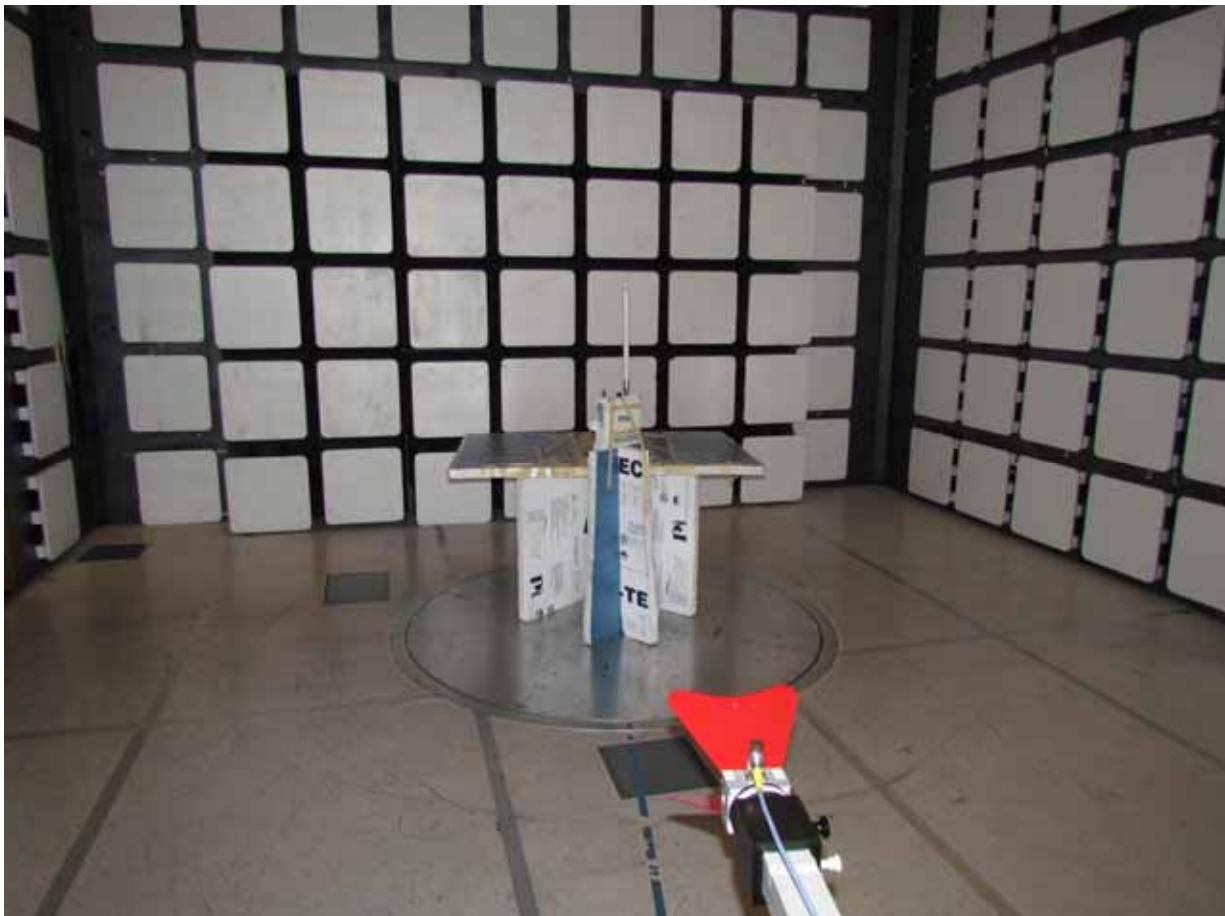
**Dynamic Frequency Selection Test Set-Up**
