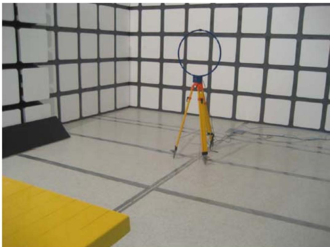
Test Configuration: 30MHz~1GHz
