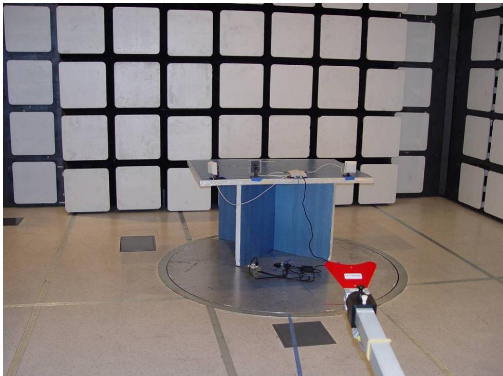
Radiated Emissions < 1GHz with Power Converter
