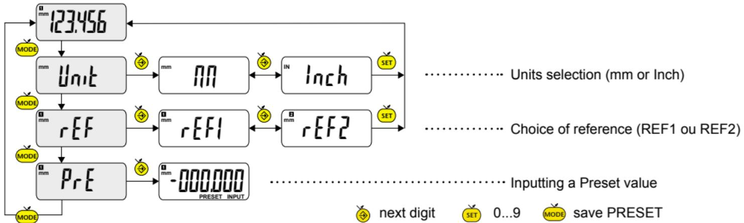
**Note:** It is possible to assign a different preset value to each of the 2 References. Similarly, different tolerance limits can be assigned to References 1 and 2.
