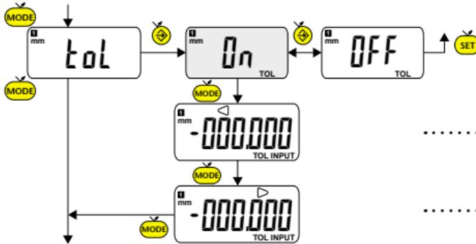
..... Input the lower tolerance limit ◀
