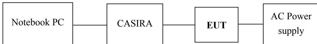
**Fig. 2-2 Ac Power Line Conduction Emission Test mode:**
