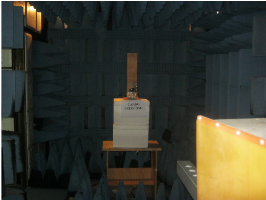
Figure 10. Radiated Emission Test Above 1GHz
