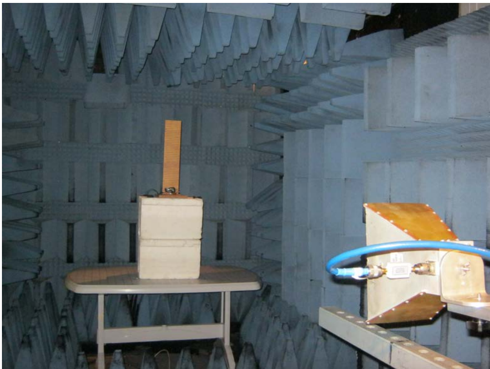
Figure 7. Radiated Emission Test, 1-18GHz
