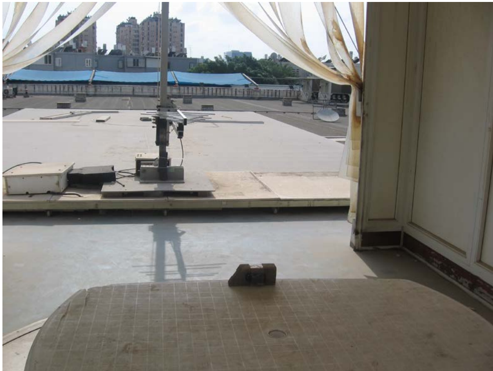
Figure 6. Radiated Emission Test, 200-1000MHz
