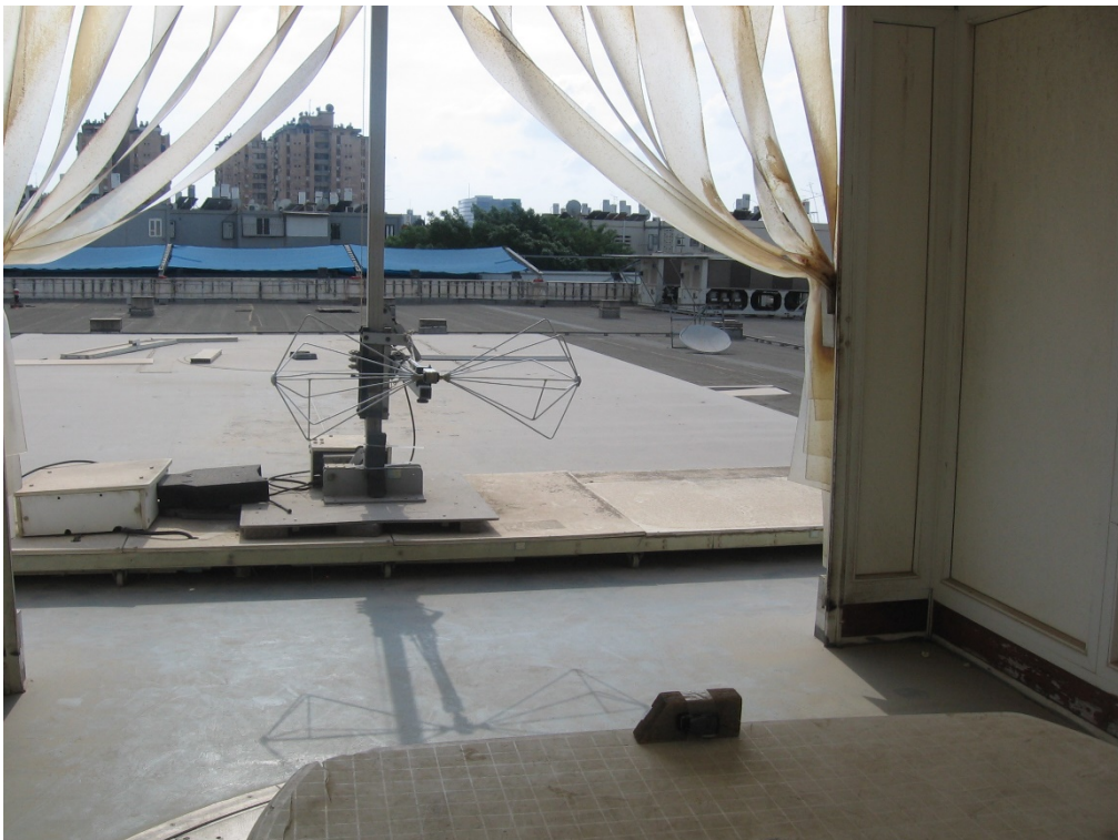
Radiated Emission Test, 30-200MHz
