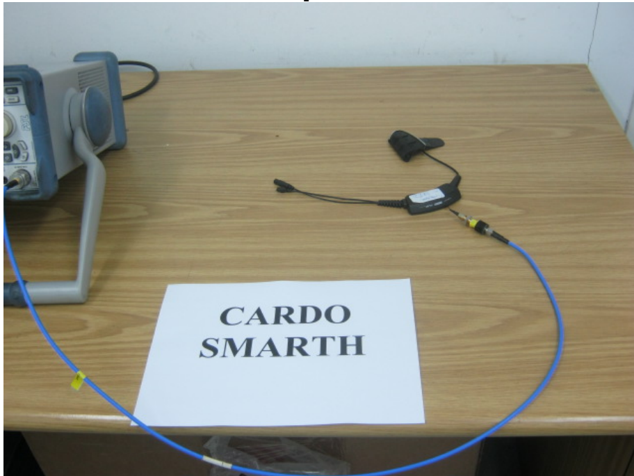
Figure 5. Conducted Emission From Antenna Ports Test
