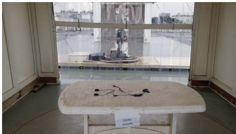
Figure 8. Radiated Emission Test
