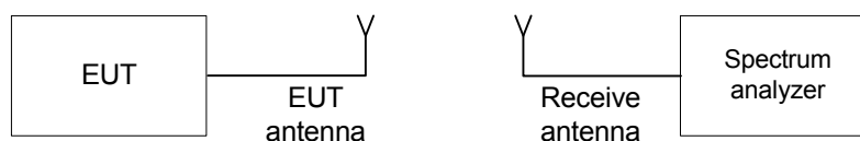
Figure 7.6.1 Band edge emission test setup
