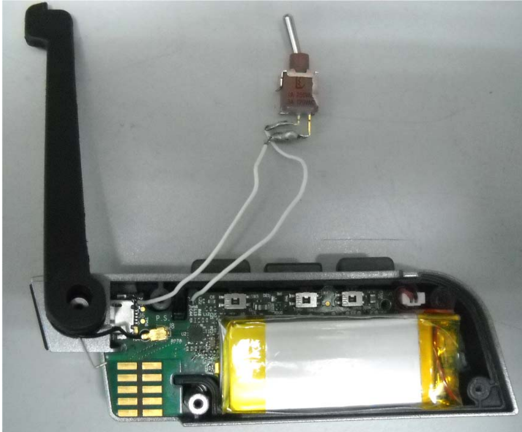
Photograph No.2 Bluetooth headset internal view
