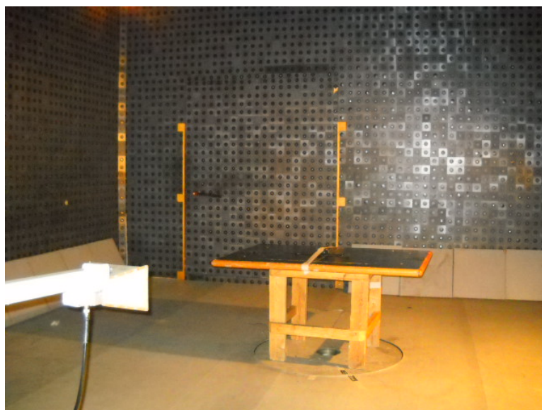
Photograph 7.2.1 Setup for carrier field strength measurements
