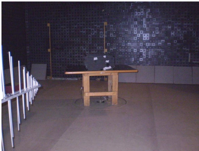
Photograph No.3 Spurious emissions field strength measurement setup in the anechoic chamber in 30 - 1000 MHz
