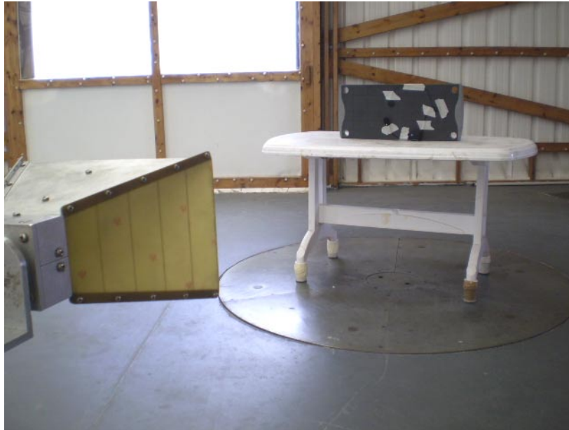
Photograph No.1 Carrier and spurious emissions field strength measurement setup at the OATS
