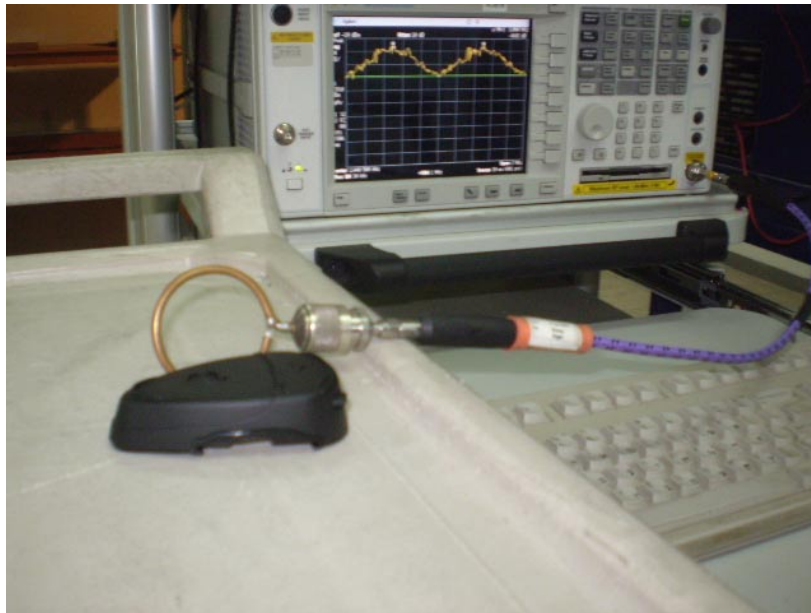
Photograph No.4 Occupied bandwidth, carrier frequency separation, number of hopping frequencies, average time of occupancy measurement setup
