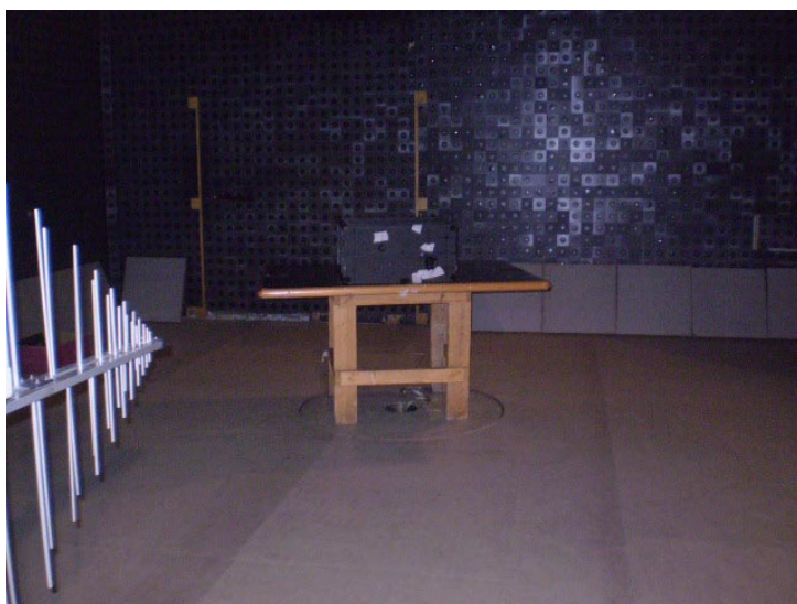
Photograph 8.1.1 Setup for radiated emission measurements
