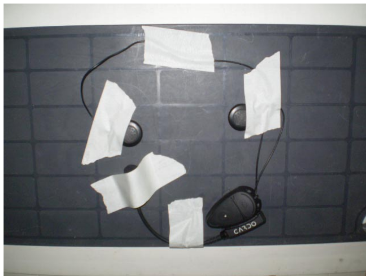
Photograph 6.6.2 EUT located on the plastic plate in vertical position (X-axis position)
