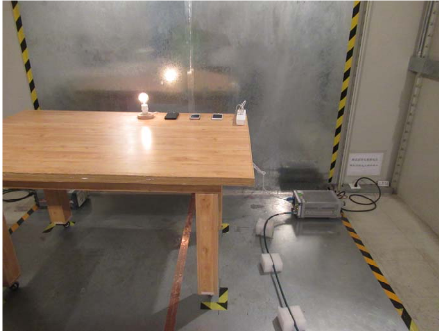
Conducted Emissions - Side View
