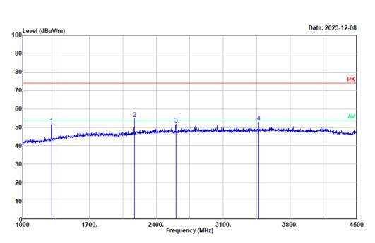
Project No. : RWAY202300007 Test Mode : Transmitting Test Voltage : DC 12V
