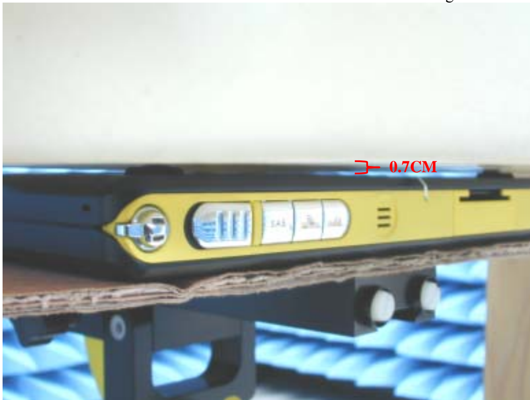
Fig.8 Photograph of the top cover parallel and at a distance of 0.0 cm from the base of the phantom(0.7 cm Spacing between EUT & Planar Phantom)
