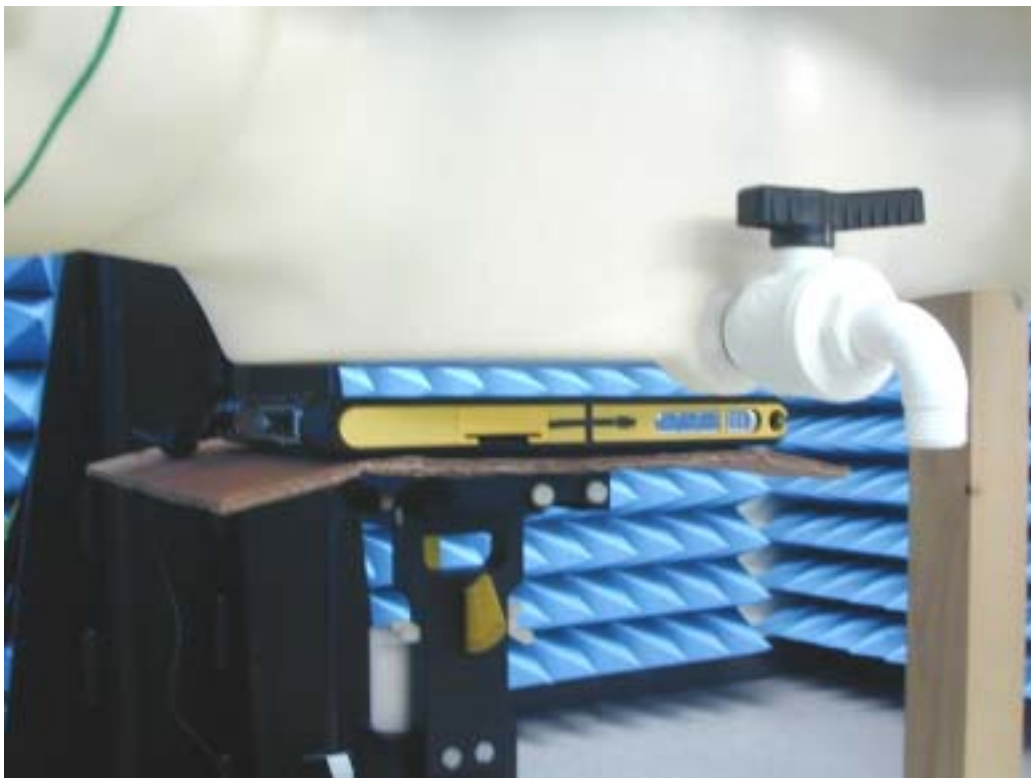
Fig.5 Photograph of the top cover parallel and at a distance of 1.5 cm from the base of the phantom
