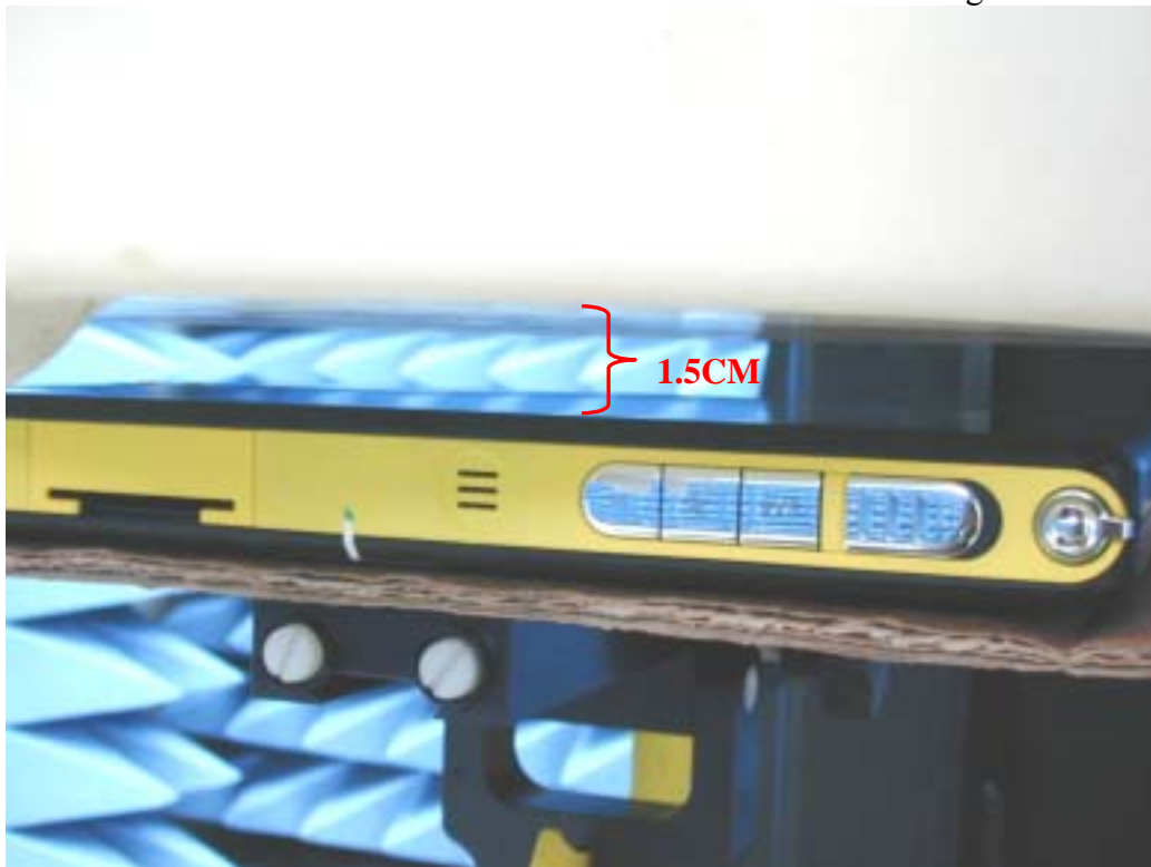
Fig.6 Photograph of the top cover parallel and at a distance of 1.5 cm from the base of the phantom
