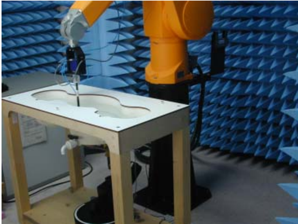
Fig.1 Photograph of the SAR measurement System
