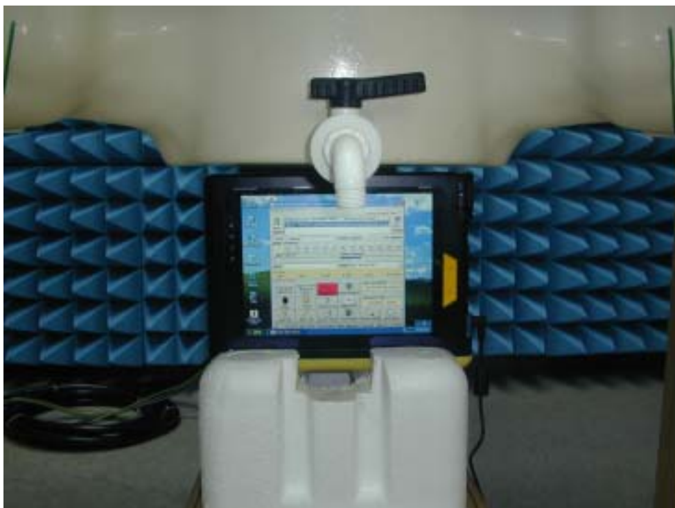
Fig.8 Photograph of the edge of the PC at 90° and at a distance of 1.5 cm from the base of the phantom
