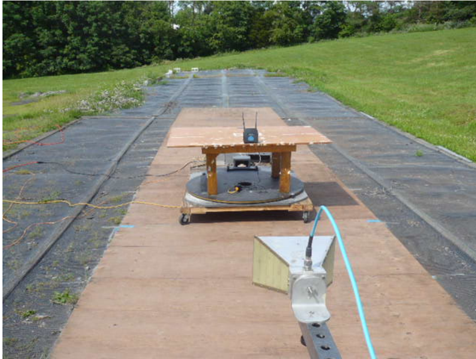
Vertical Antenna Polarization
