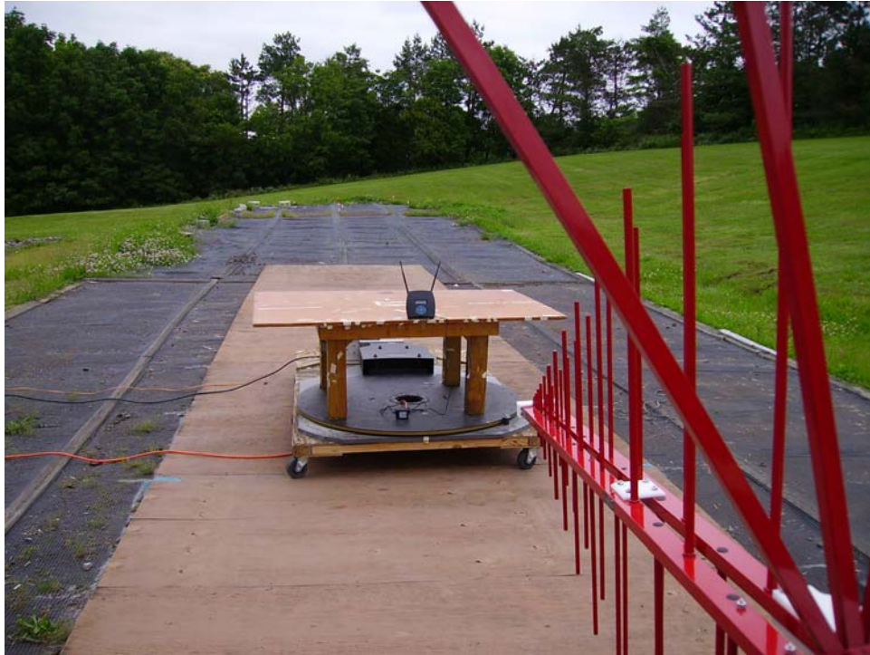
Vertical Antenna Polarization
