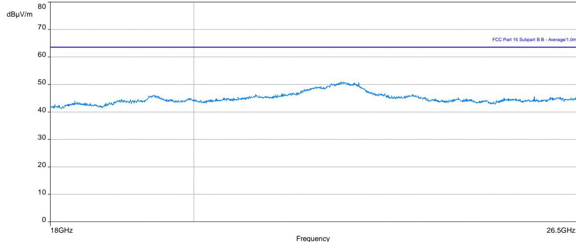
Note: testing was performed to 40 GHz, no emissions above 26.5 GHz were detected and the reading were below the applicable limit(s).
