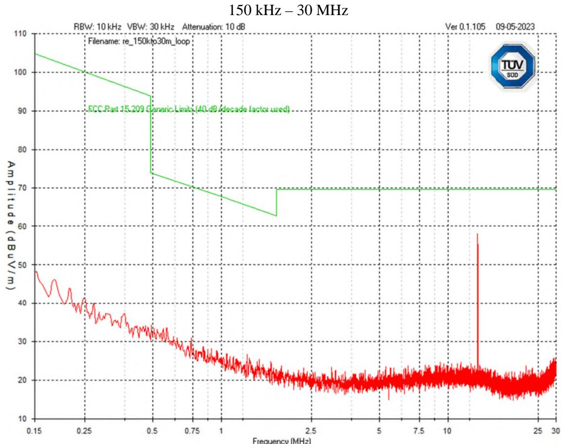
Note: Spike shown at 13.56 MHz is intentional RFID signal.
