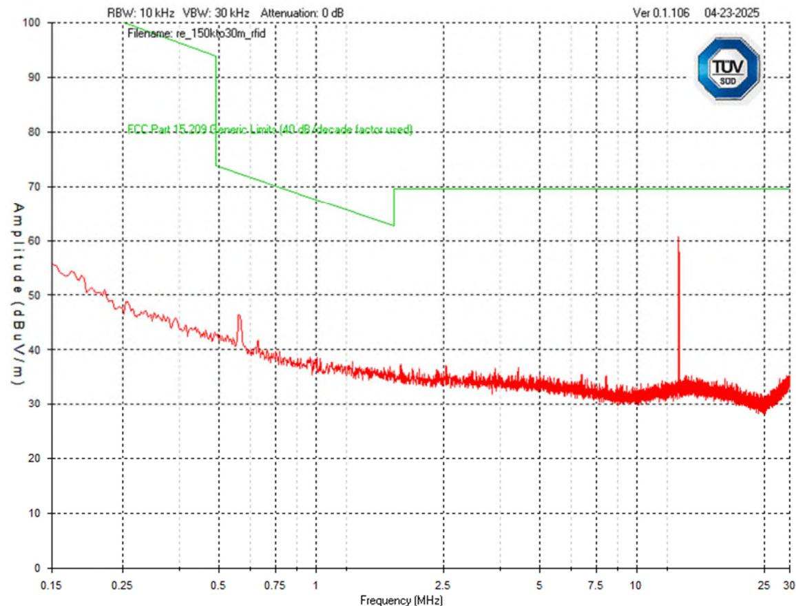
Note: Spike shown at 13.56 MHz is intentional RFID signal. Device was scanned down to 9 kHz, no emissions were detected below 150 kHz and the emissions were below the limit.
