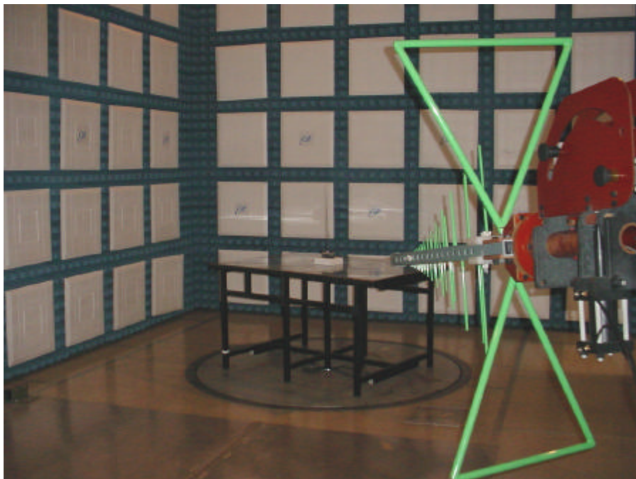
TEST SETUP FOR RADIATED EMISSIONS MEASUREMENTS MAXIMIZED FOR MEASUREMENT OF WORST CASE EMISSIONS VERTICAL POLARIZATION
