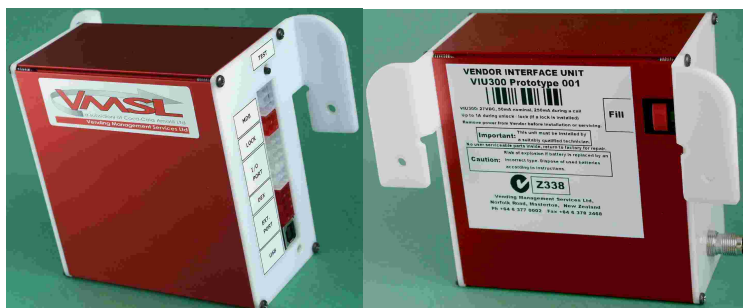
Connector locations on VIU300 Unit
