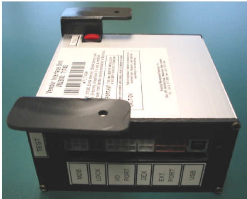
Vendor Interface Unit, Model VIU300: 71740 - Left Side View, Showing Connectors
