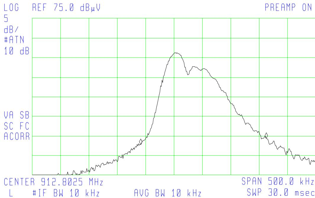
Bandwidth 99% power = 221.3 kHz. EUT emission is contained wholly in the band 902-928 MHz.
