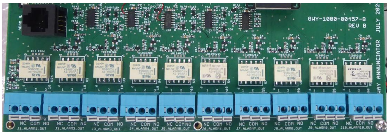
Figure 24: Annunciator Dry Contact Connector for Alarming
