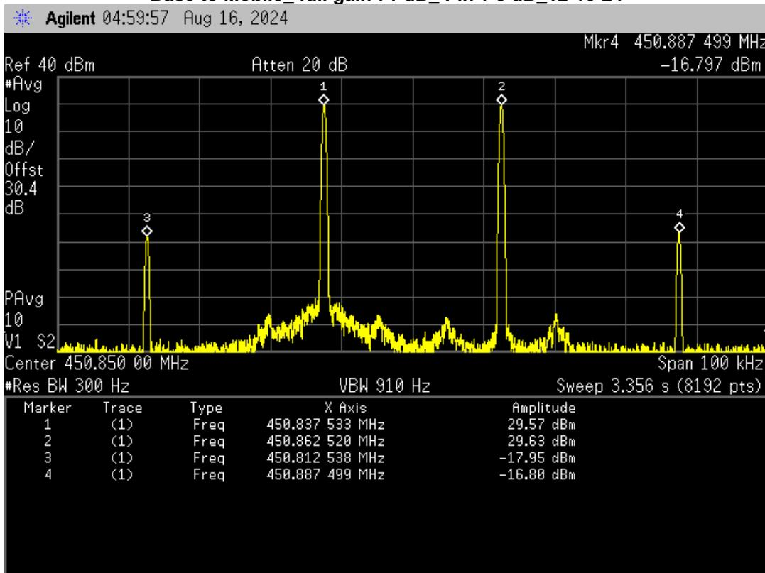
**Mobile to Base\_ full gain 72 dB\_ Pin -44.0 dBm\_12-10-24**
