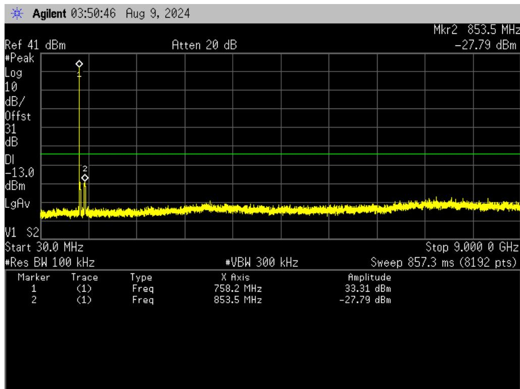
758 – 775 MHz\_ Test Freq = 766 MHz
