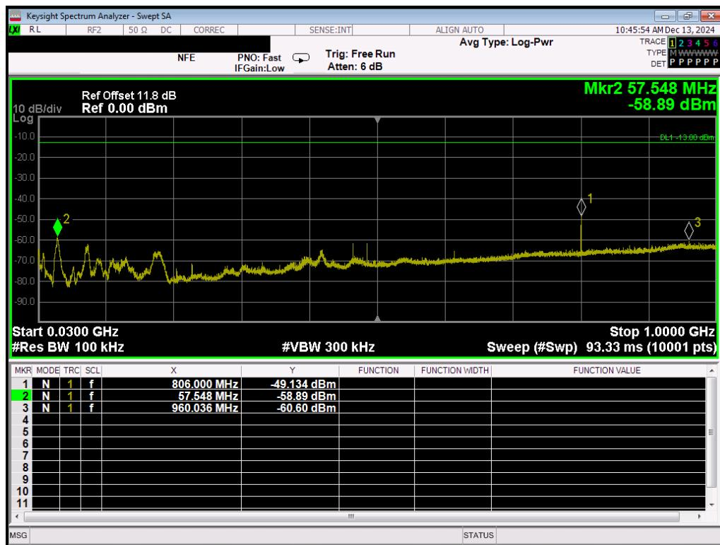
Mobile to Base\_1 - 9 GHz\_ Test Freq = 806 MHz
