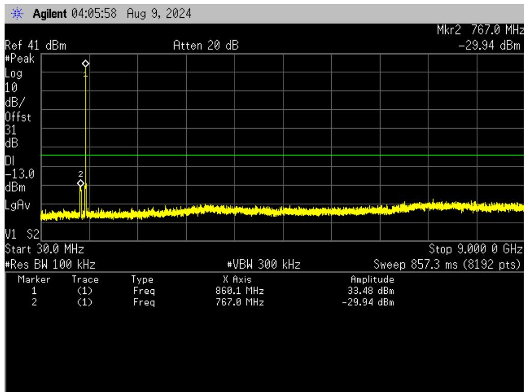
851 - 869 MHz\_ Test Freq = 869 MHz
