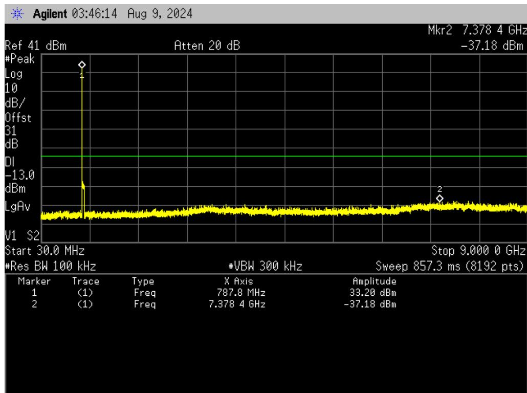
788 - 824 MHz\_ Test Freq = 806 MHz
