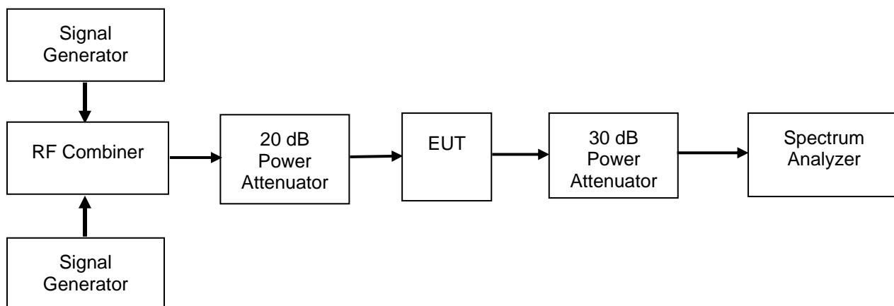
**Booster Intermodulation at 0.2 dB below AGC Threshold**
