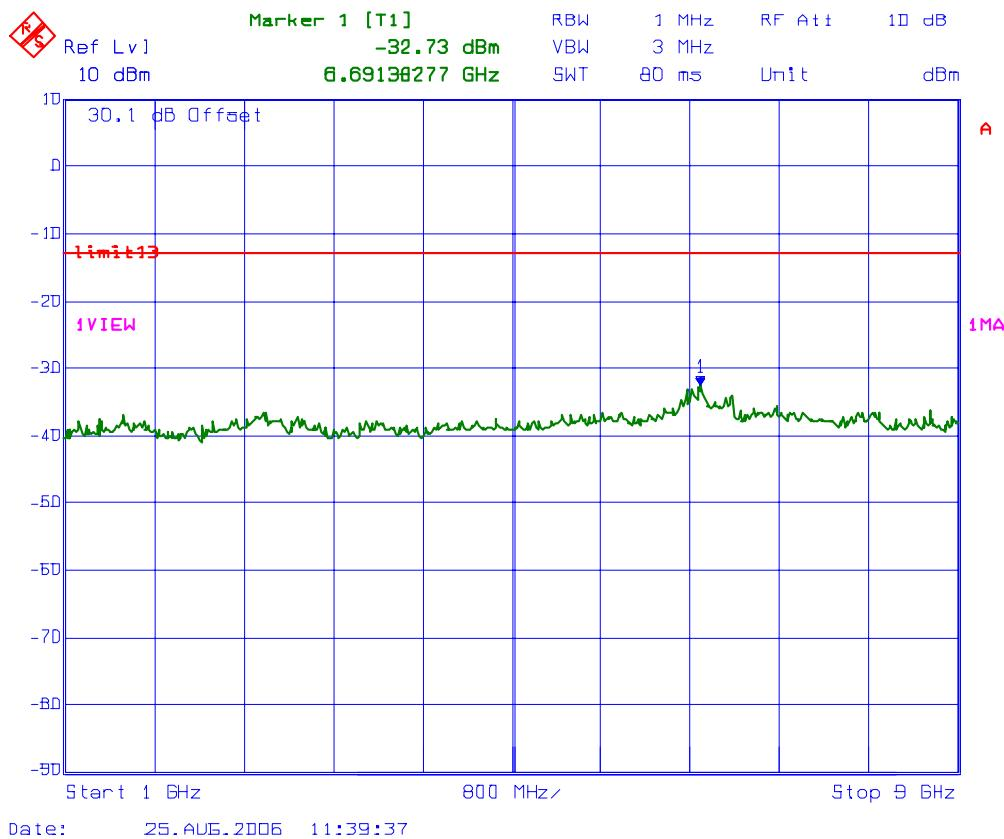
**PLOT # 89    Antenna Conducted RF Spurious Emissions @ Fc: 794 MHz**
