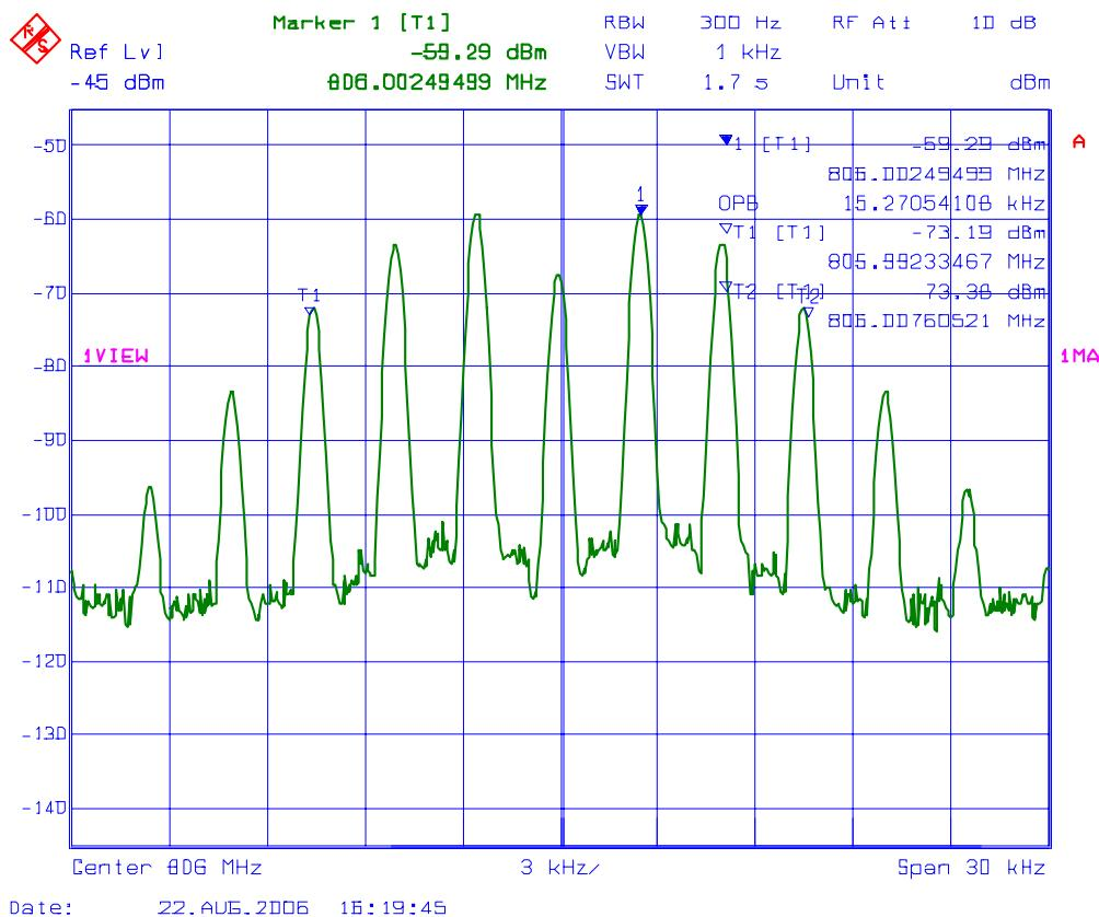
**PLOT # 46** 99% Occupied Bandwidth – RF Output Signal
