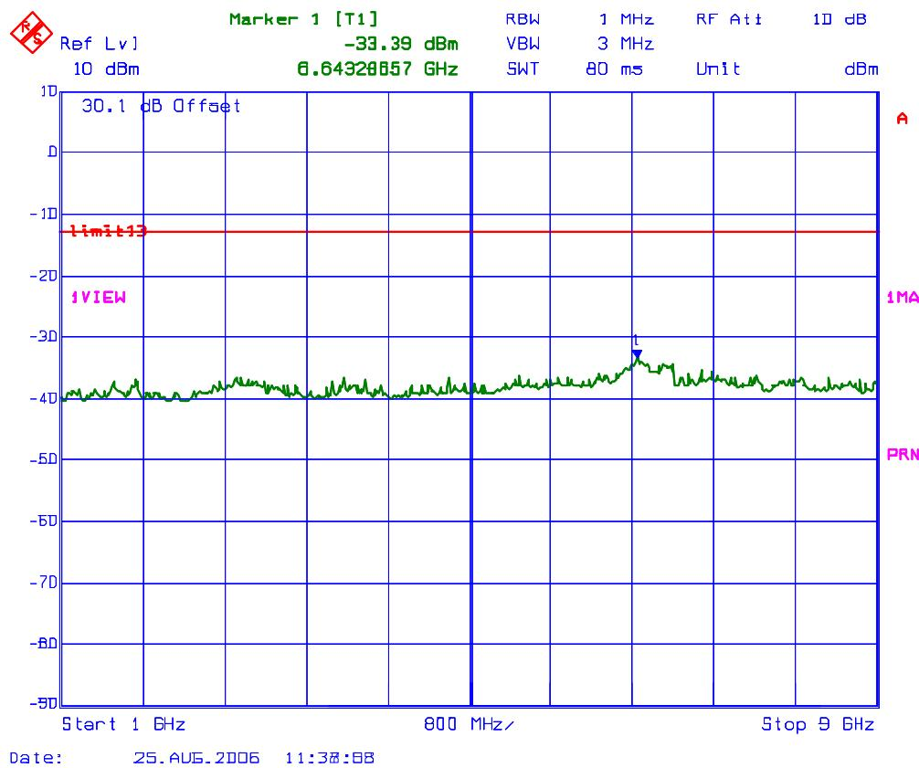
**PLOT # 101 Antenna Conducted RF Spurious Emissions @ Fc: 860 MHz**
