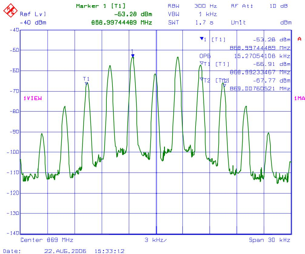
**PLOT # 76** 99% Occupied Bandwidth – RF Output Signal
