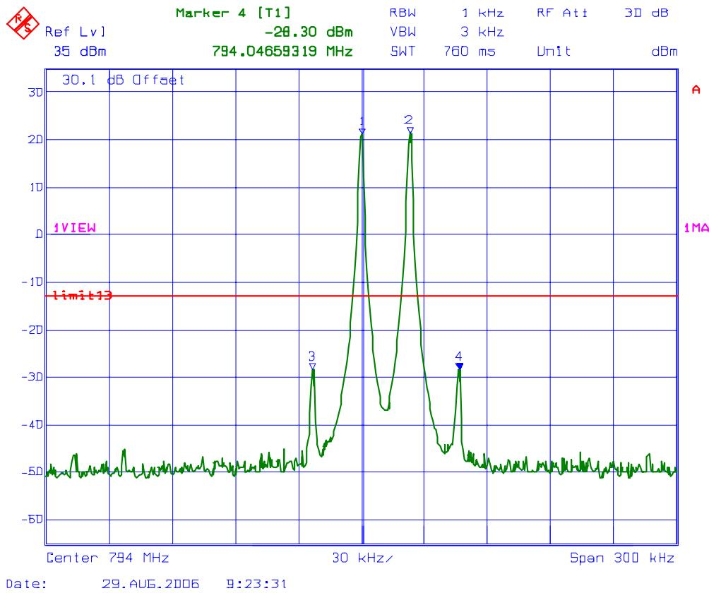
**PLOT #: 5 Intermodulation with 3 RF signal inputs/outputs**
