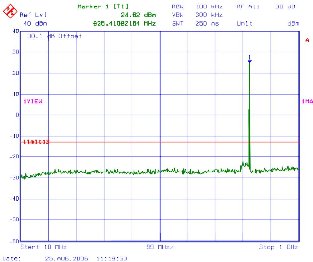
**PLOT # 98    Antenna Conducted RF Spurious Emissions @ Fc: 824 MHz**
