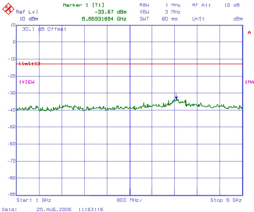
**PLOT # 97 Antenna Conducted RF Spurious Emissions @ Fc: 824 MHz**
