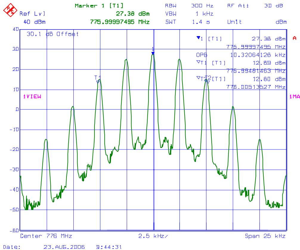
**PLOT # 25 99% Occupied Bandwidth – RF Input Signal**
