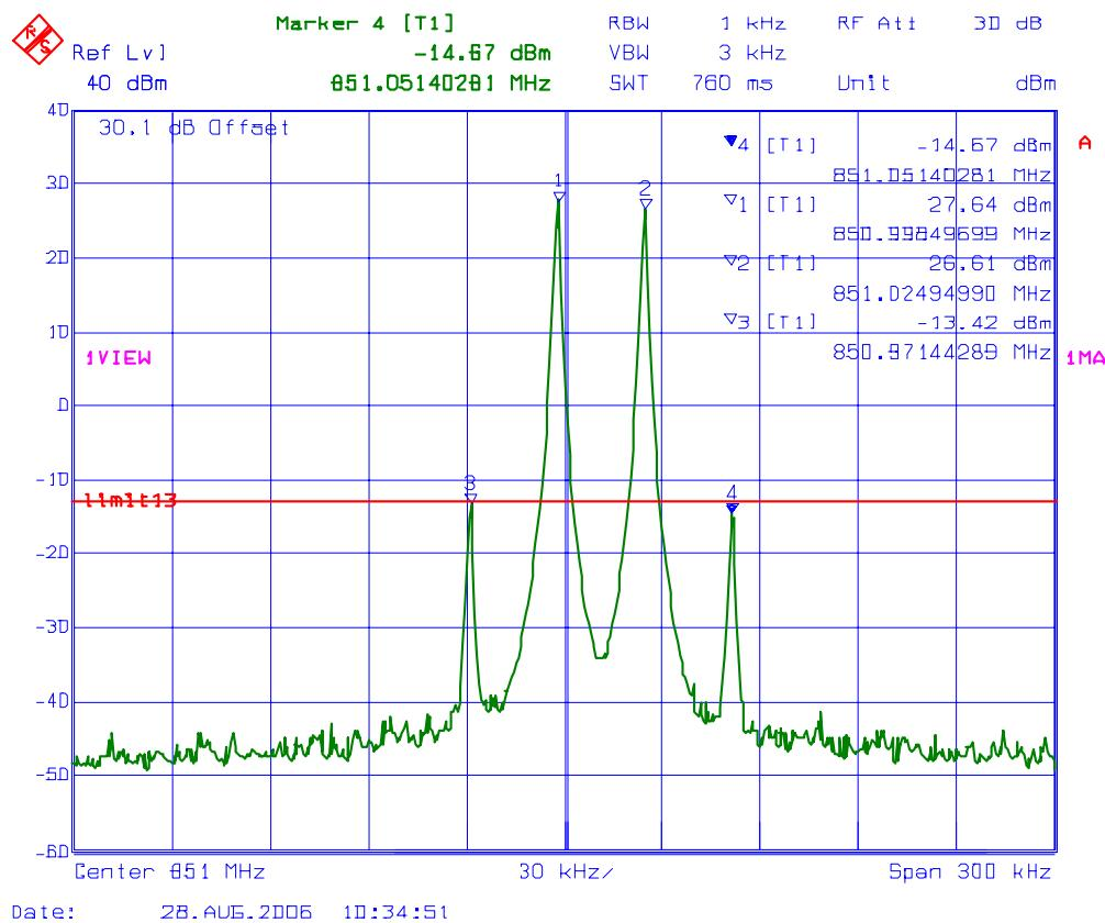
**PLOT #: 11** Intermodulation with 3 RF signal inputs/outputs
