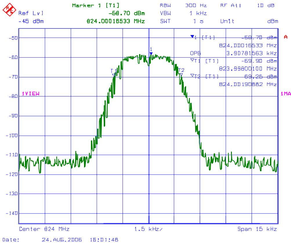
**PLOT # 58 99% Occupied Bandwidth – RF Output Signal**
