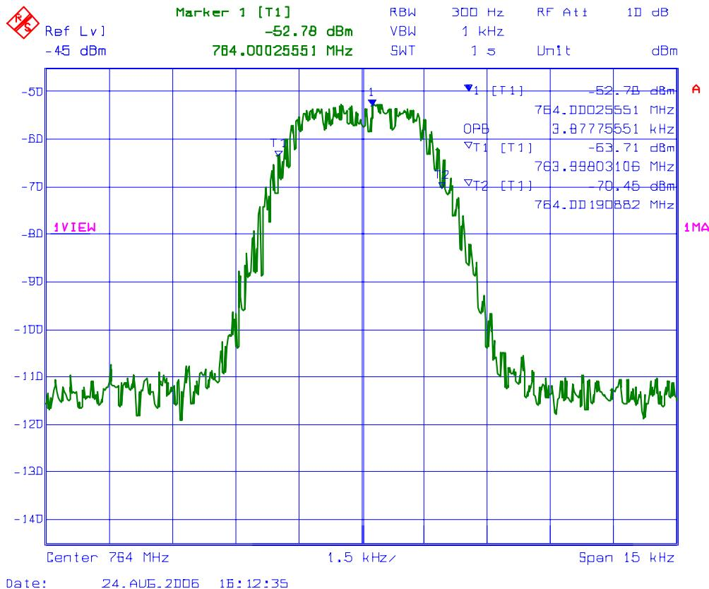
**PLOT # 18 99% Occupied Bandwidth – RF Output Signal**
