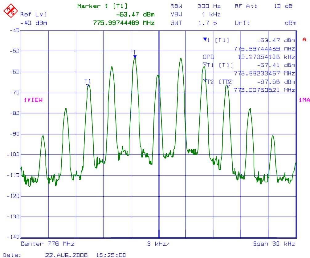
**PLOT # 26** 99% Occupied Bandwidth – RF Output Signal
