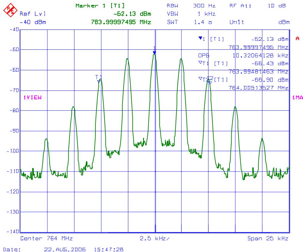
**PLOT # 14** 99% Occupied Bandwidth – RF Output Signal
