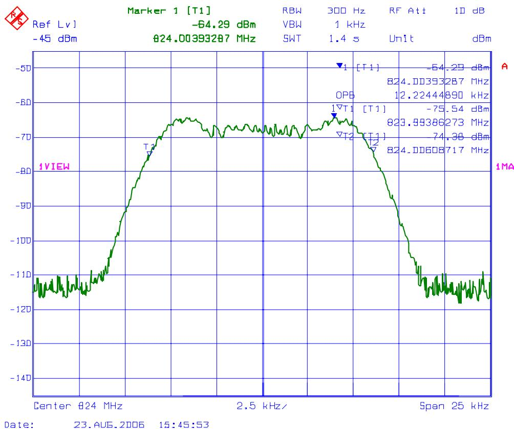
**PLOT # 62 99% Occupied Bandwidth – RF Output Signal**
