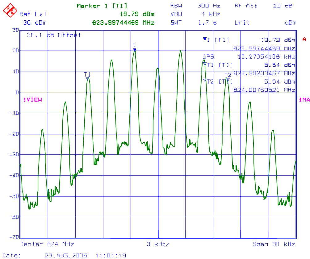
**PLOT # 57 99% Occupied Bandwidth – RF Input Signal**
