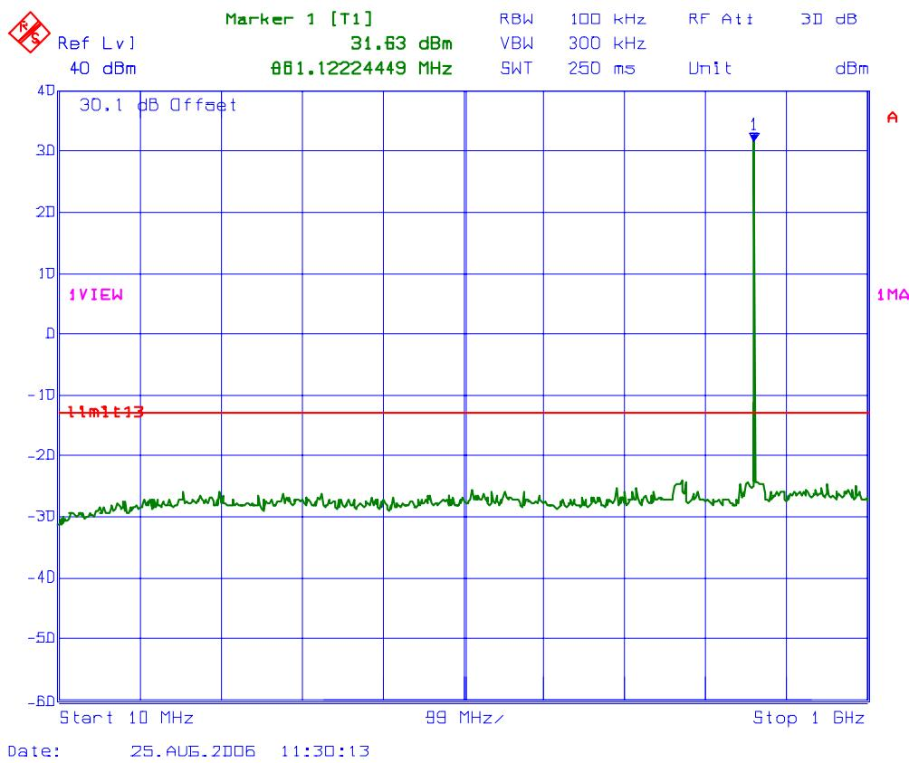
**PLOT # 102 Antenna Conducted RF Spurious Emissions @ Fc: 860 MHz**
