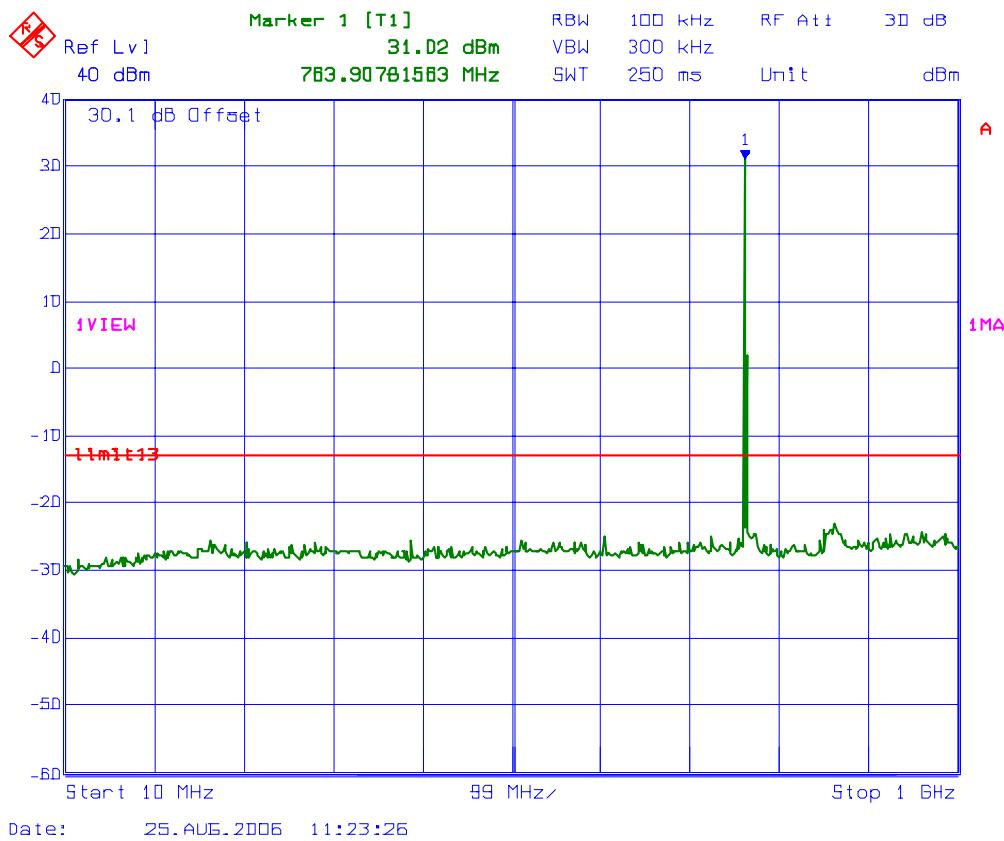
**PLOT # 84 Antenna Conducted RF Spurious Emissions @ Fc: 764 MHz**
