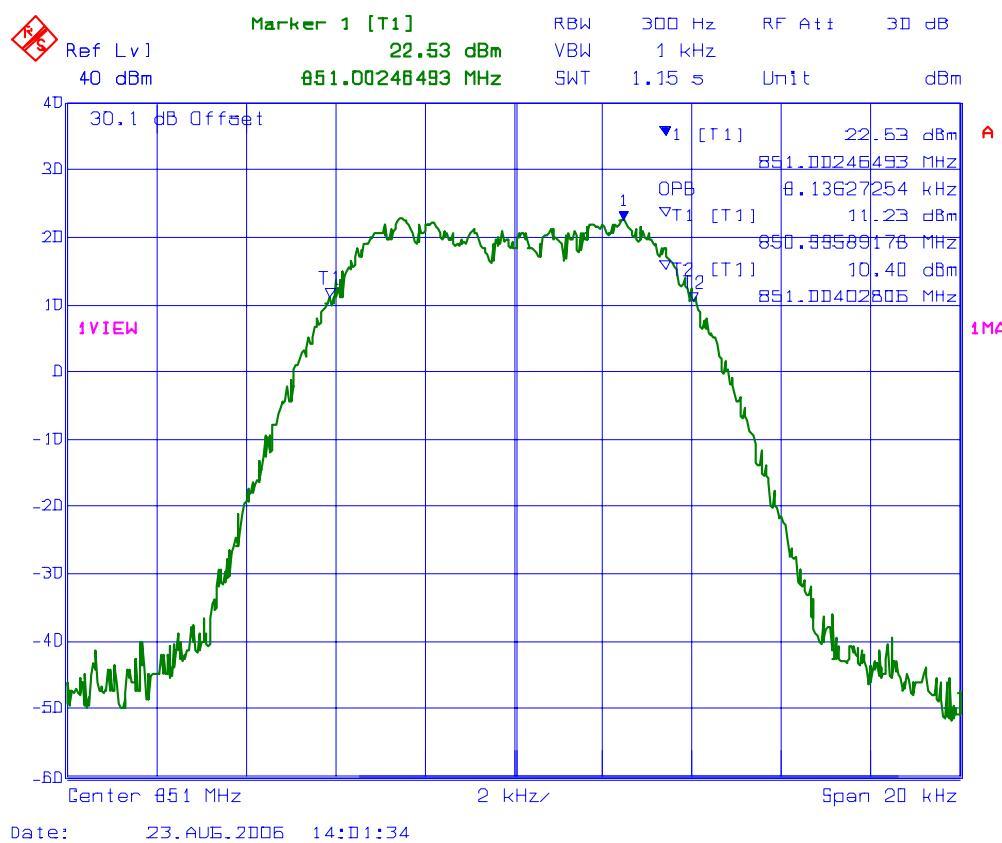
**PLOT # 71 99% Occupied Bandwidth – RF Input Signal**
