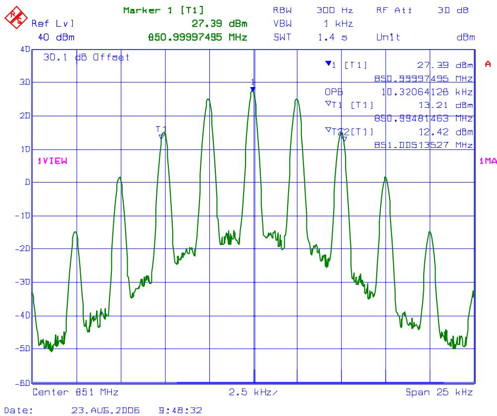
**PLOT # 65 99% Occupied Bandwidth – RF Input Signal**
