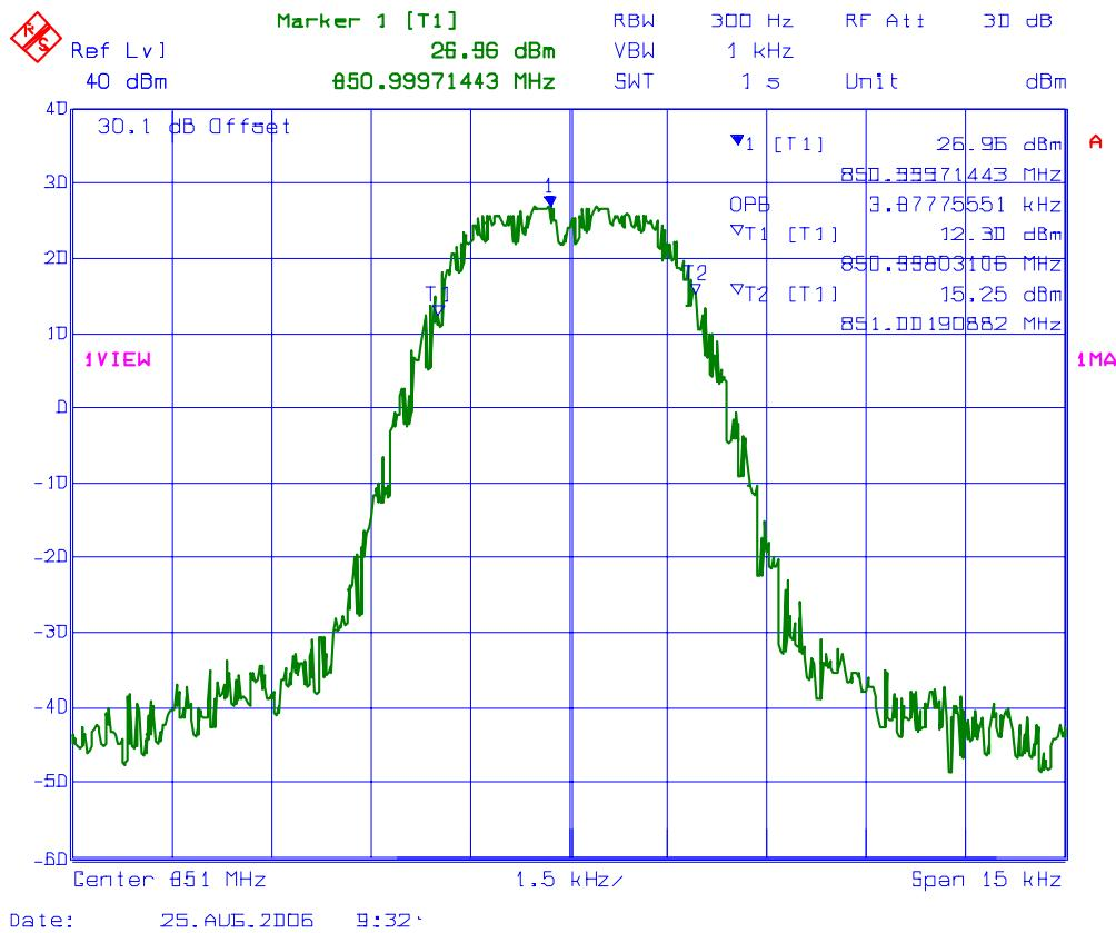
**PLOT # 69 99% Occupied Bandwidth – RF Input Signal**
