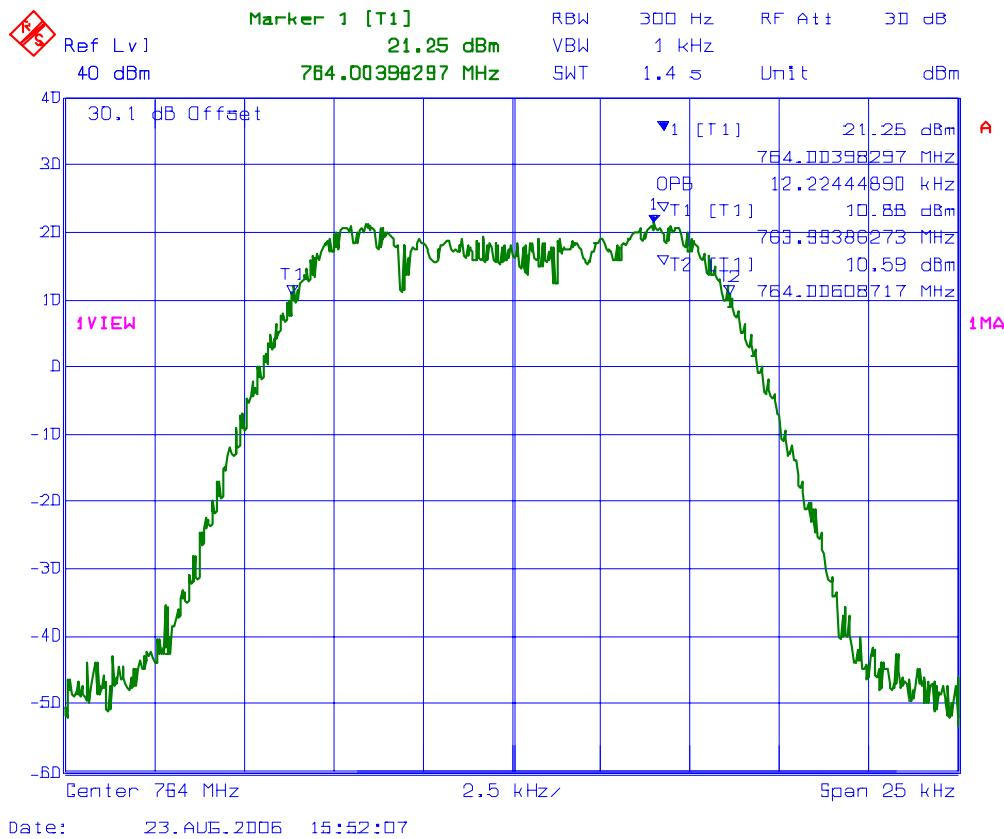
**PLOT # 23 99% Occupied Bandwidth – RF Input Signal**
