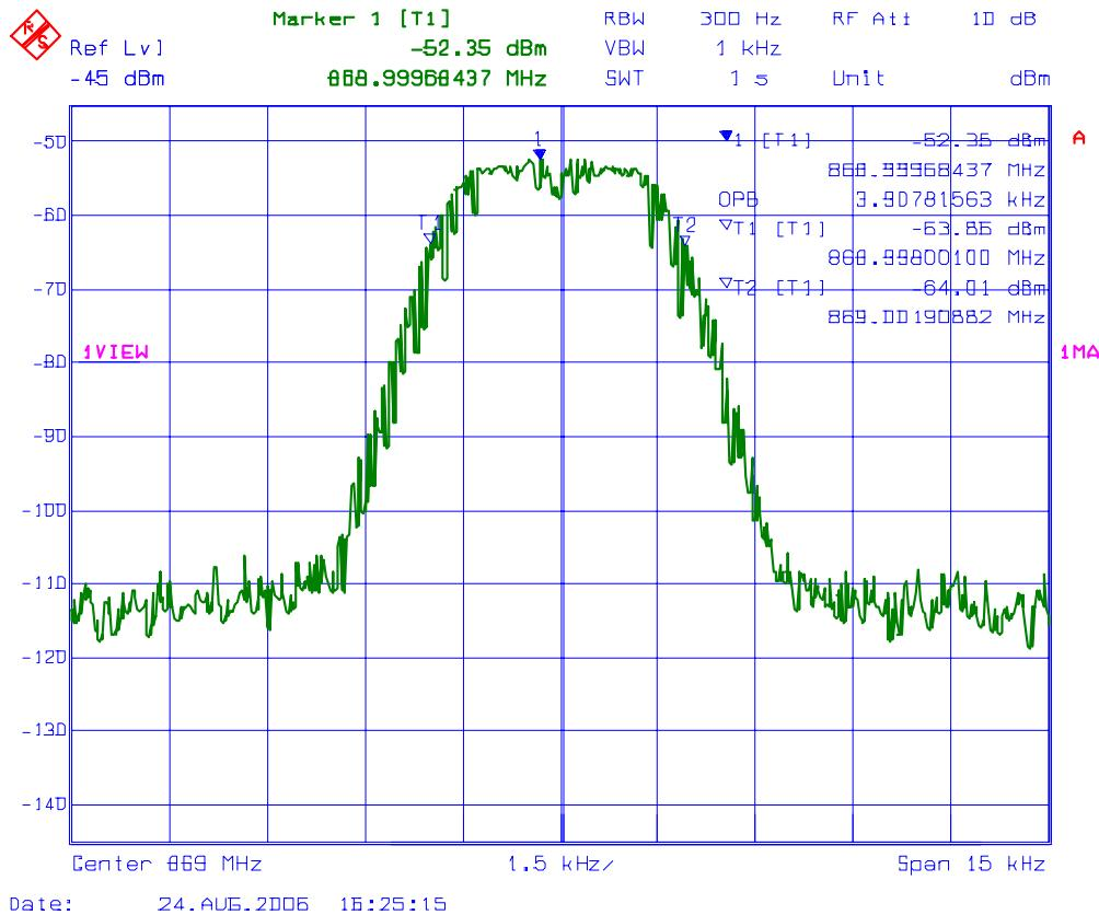
**PLOT # 78** 99% Occupied Bandwidth – RF Output Signal
