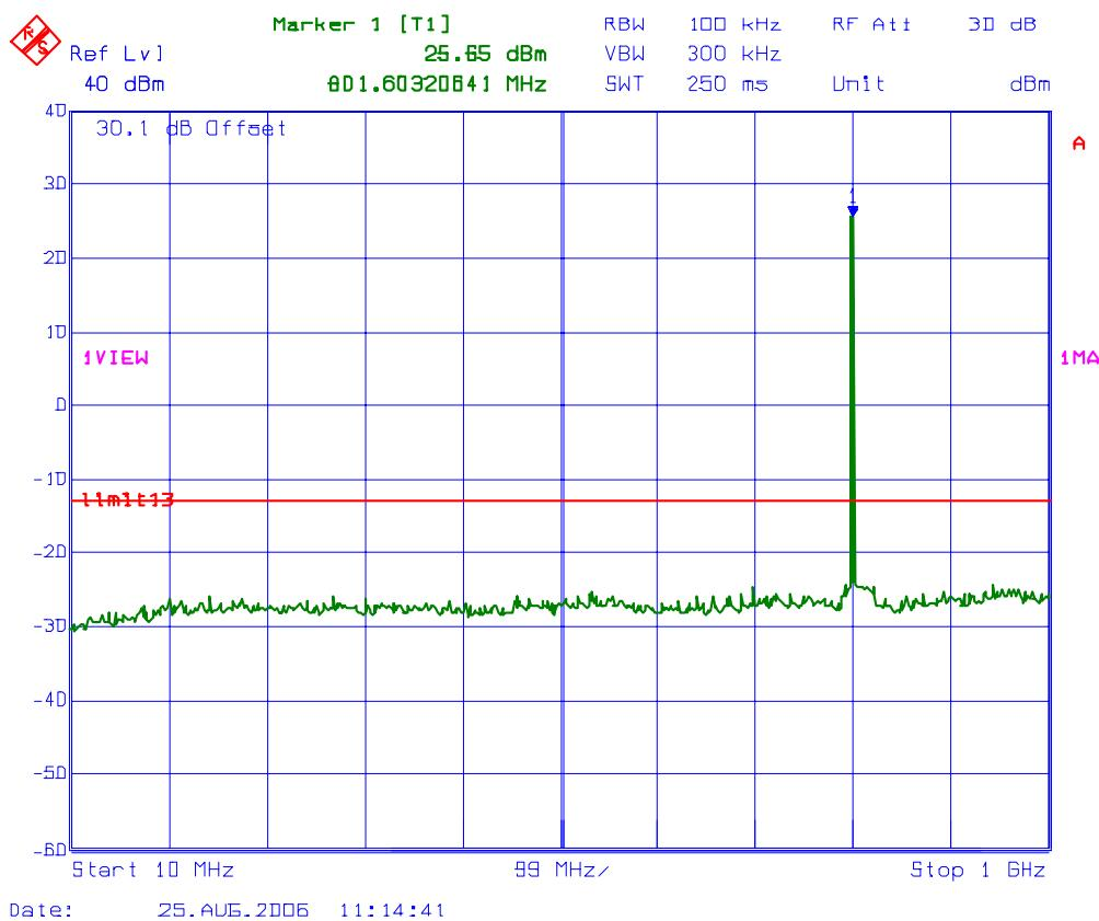
**PLOT # 92 Antenna Conducted RF Spurious Emissions @ Fc: 800 MHz**
