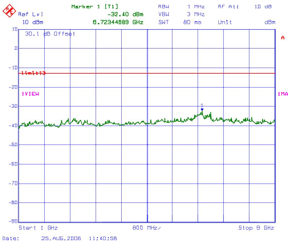
PLOT # 87 Antenna Conducted RF Spurious Emissions @ Fc: 776 MHz
