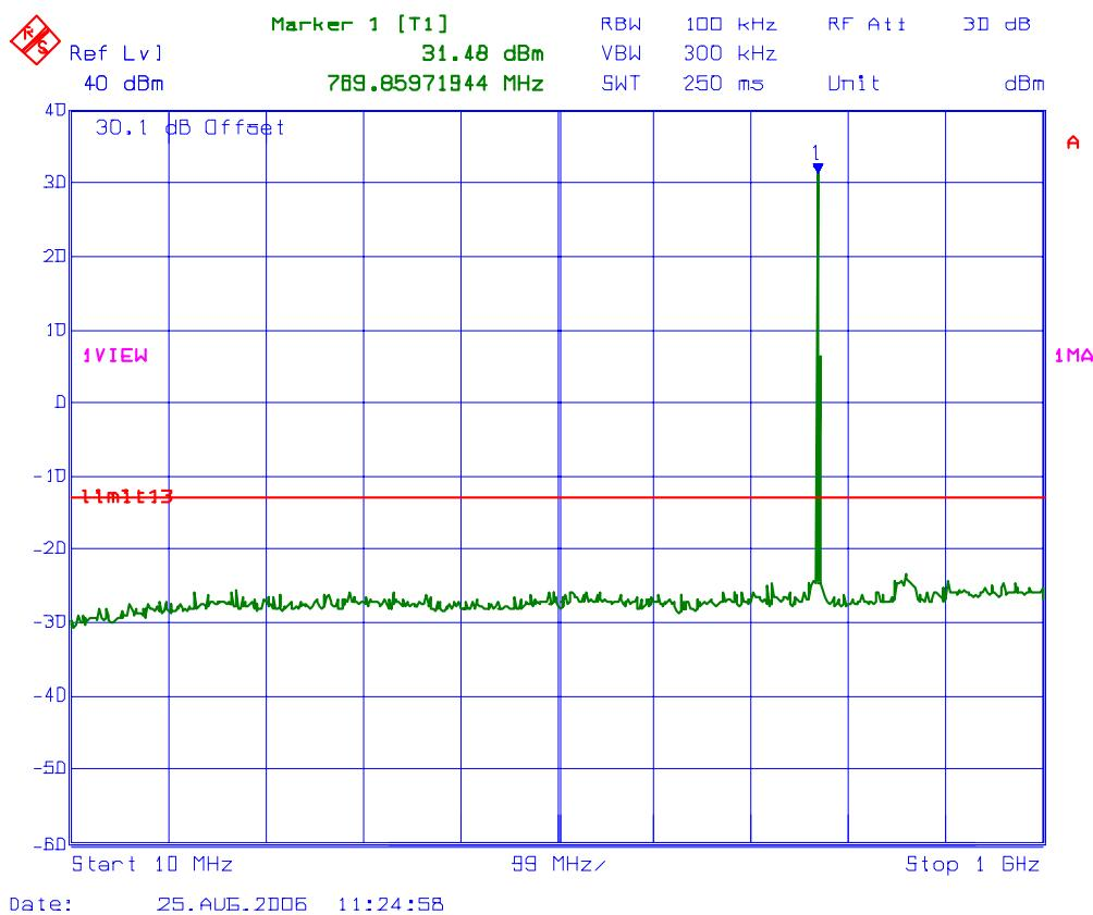
**PLOT # 86    Antenna Conducted RF Spurious Emissions @ Fc: 770 MHz**
