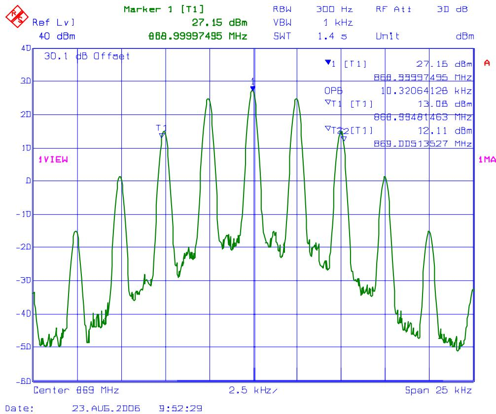
**PLOT # 75 99% Occupied Bandwidth – RF Input Signal**
