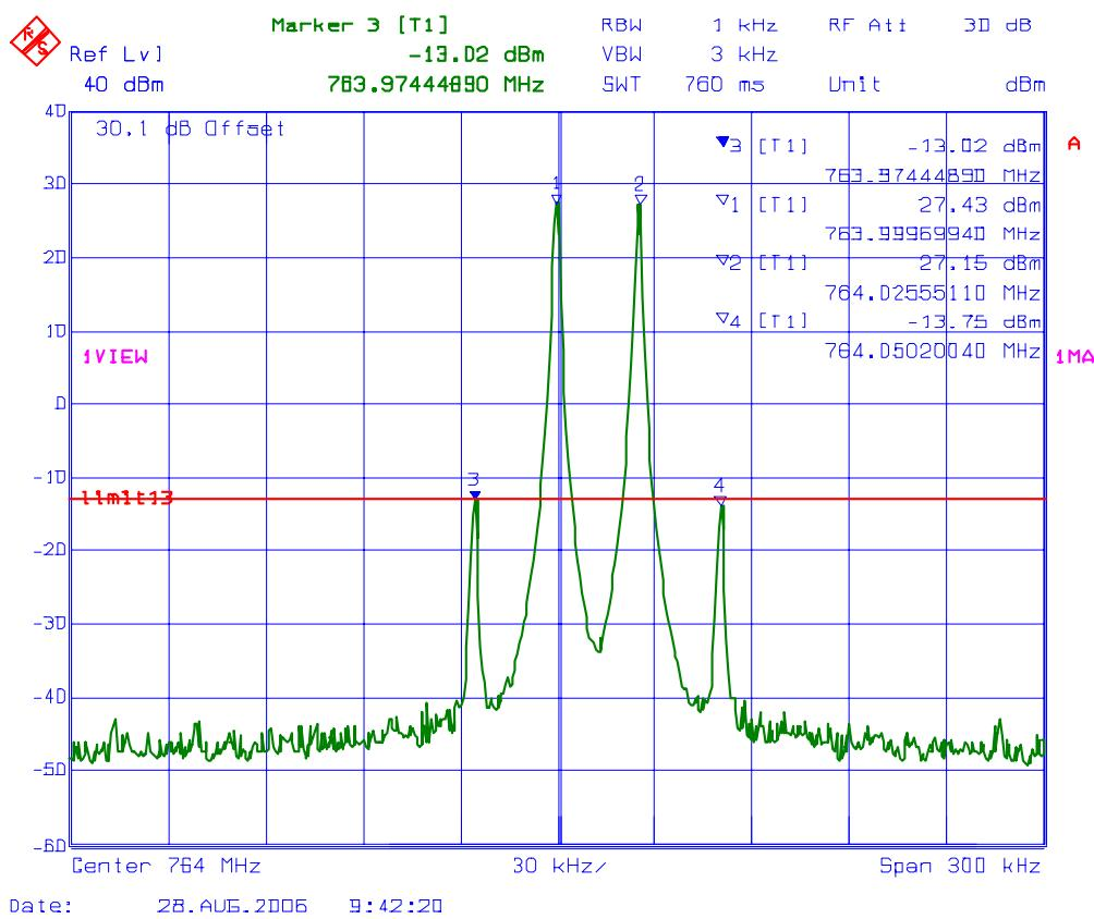
**PLOT #:** 2 **Intermodulation with 3 RF signal inputs/outputs**
