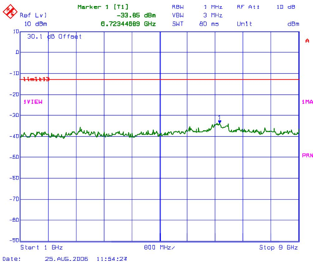
PLOT # 99 Antenna Conducted RF Spurious Emissions @ Fc: 851 MHz
