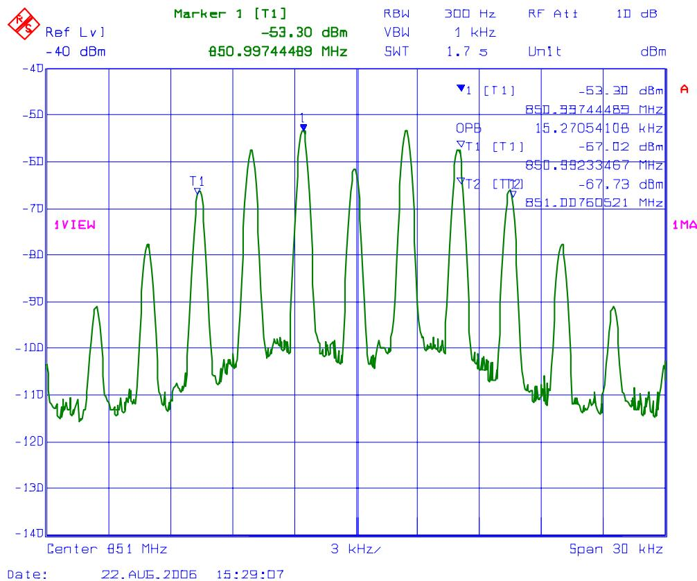
**PLOT # 66 99% Occupied Bandwidth – RF Output Signal**
