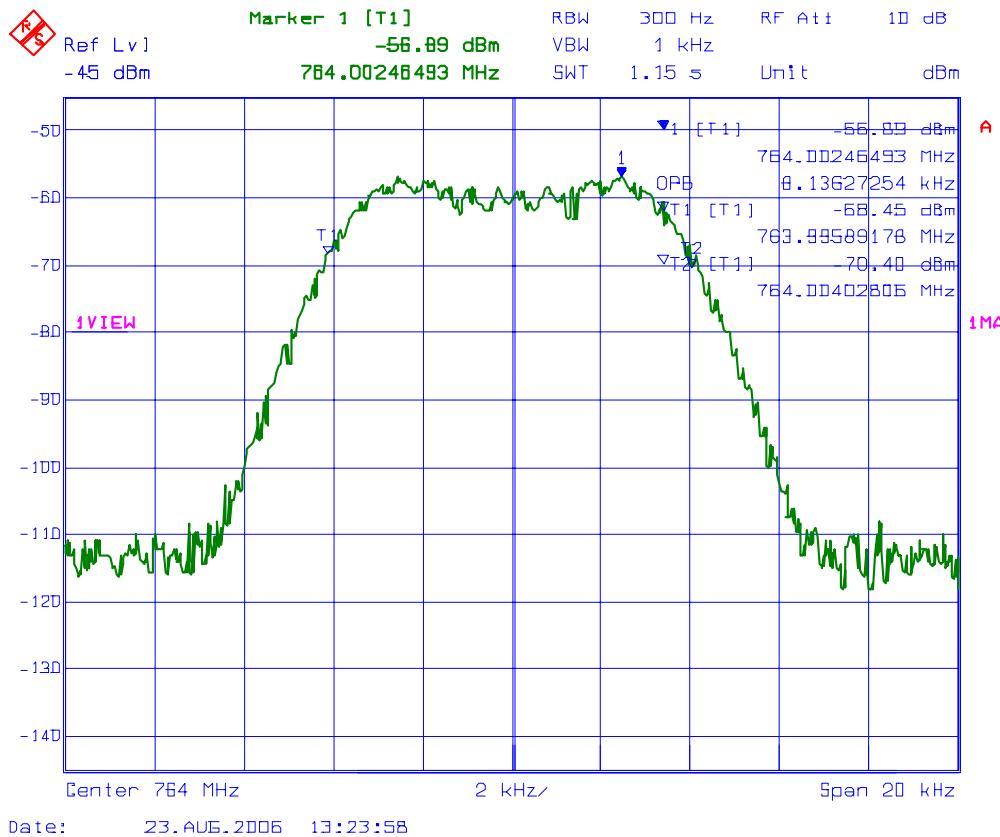
**PLOT # 20 99% Occupied Bandwidth – RF Output Signal**
