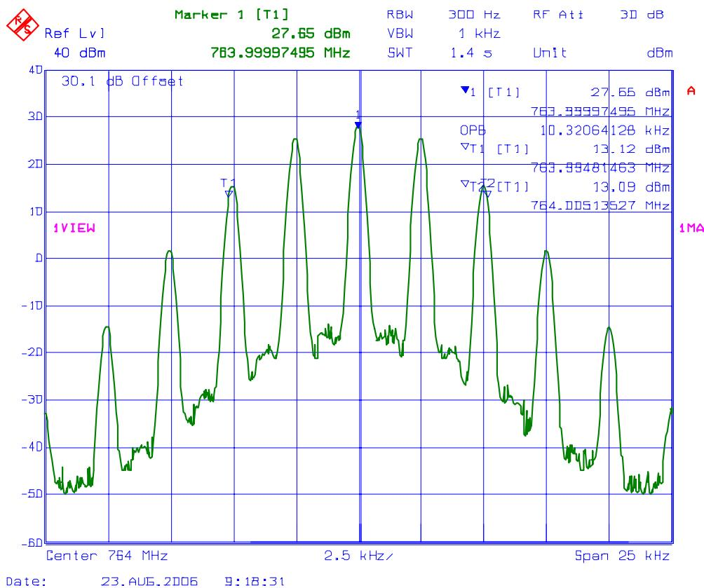
**PLOT # 15 99% Occupied Bandwidth – RF Input Signal**
