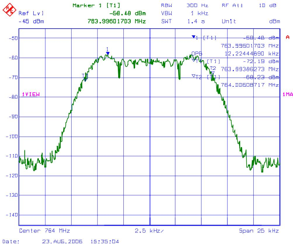
**PLOT # 22 99% Occupied Bandwidth – RF Output Signal**
