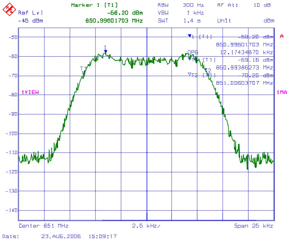
**PLOT # 72** 99% Occupied Bandwidth – RF Output Signal
