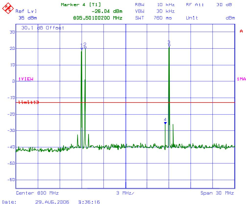
**PLOT #: 6 Intermodulation with 2 RF signal inputs/outputs**
