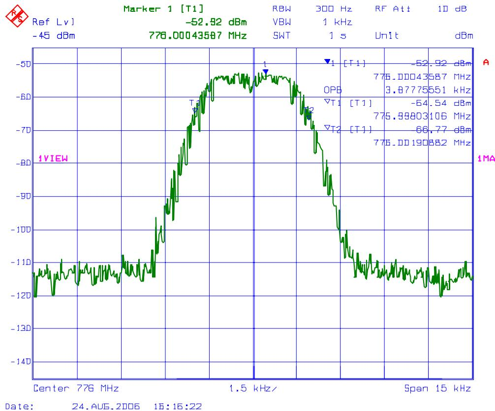
**PLOT # 28** 99% Occupied Bandwidth – RF Output Signal
