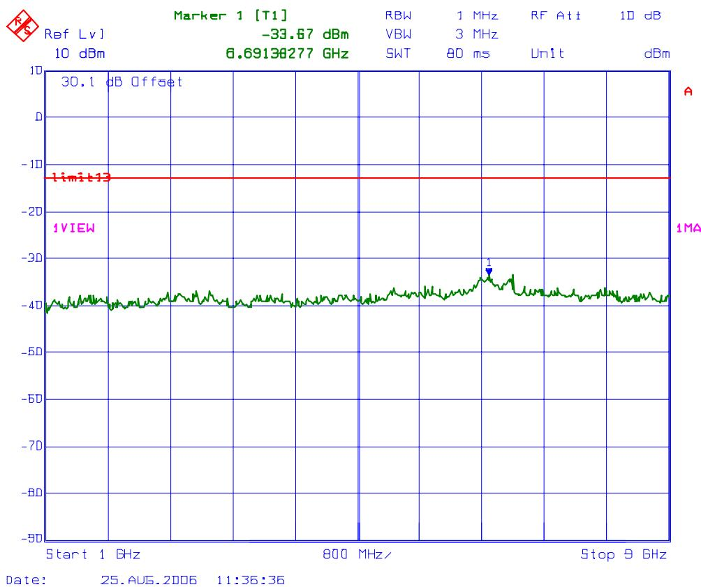
**PLOT # 103 Antenna Conducted RF Spurious Emissions @ Fc: 869 MHz**
