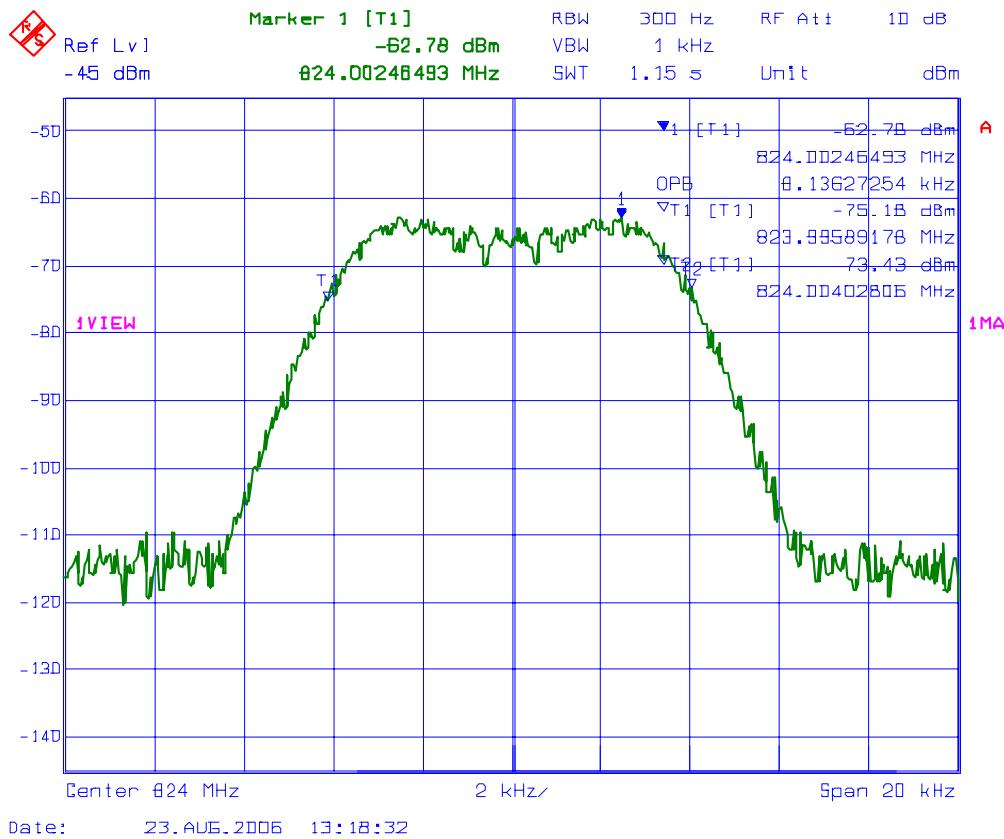
**PLOT # 60 99% Occupied Bandwidth – RF Output Signal**
