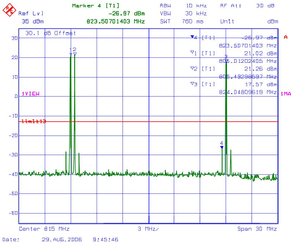
**PLOT #: 9** **Intermodulation with 2 RF signal inputs/outputs**
