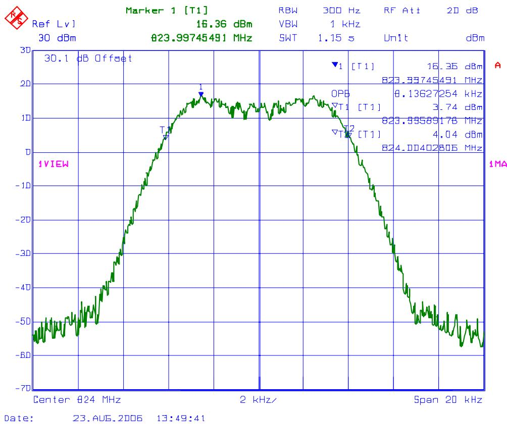
**PLOT # 61 99% Occupied Bandwidth – RF Input Signal**
