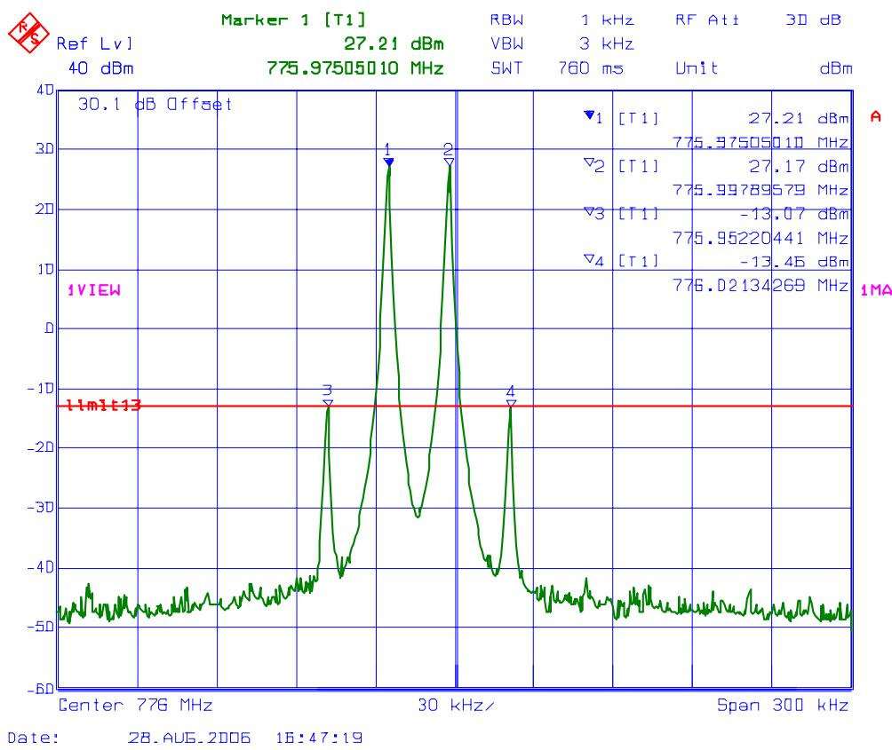
**PLOT #: 4** **Intermodulation with 2 RF signal inputs/outputs**
