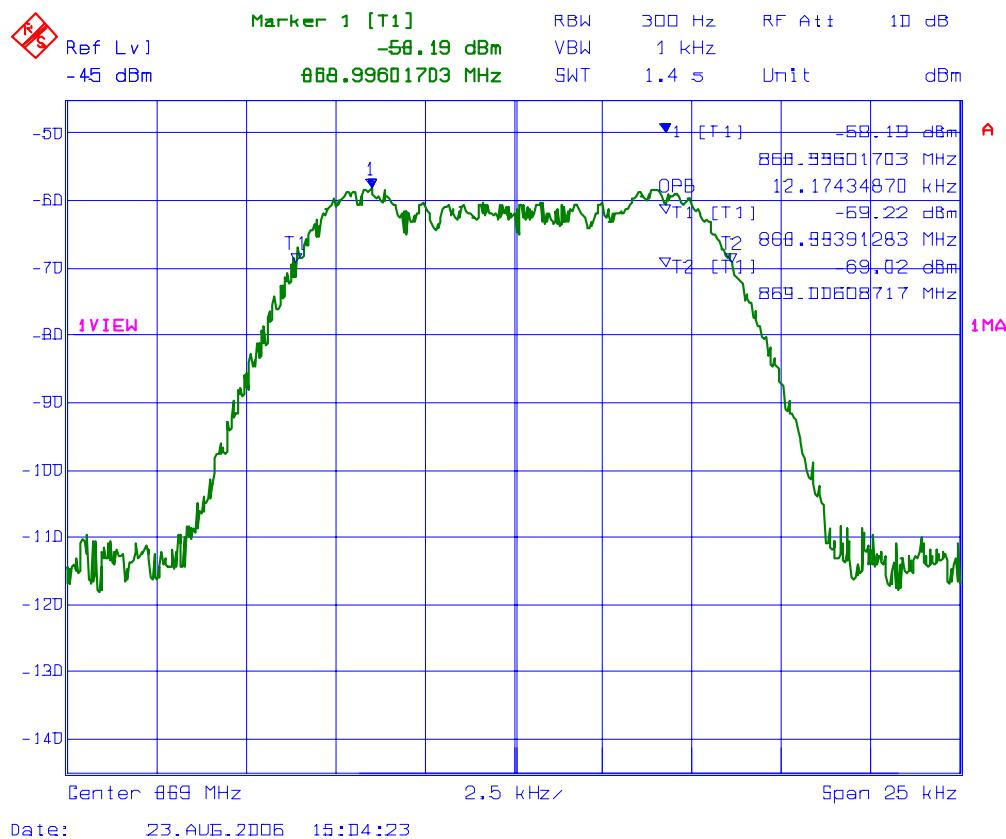
**PLOT # 82 99% Occupied Bandwidth – RF Output Signal**
