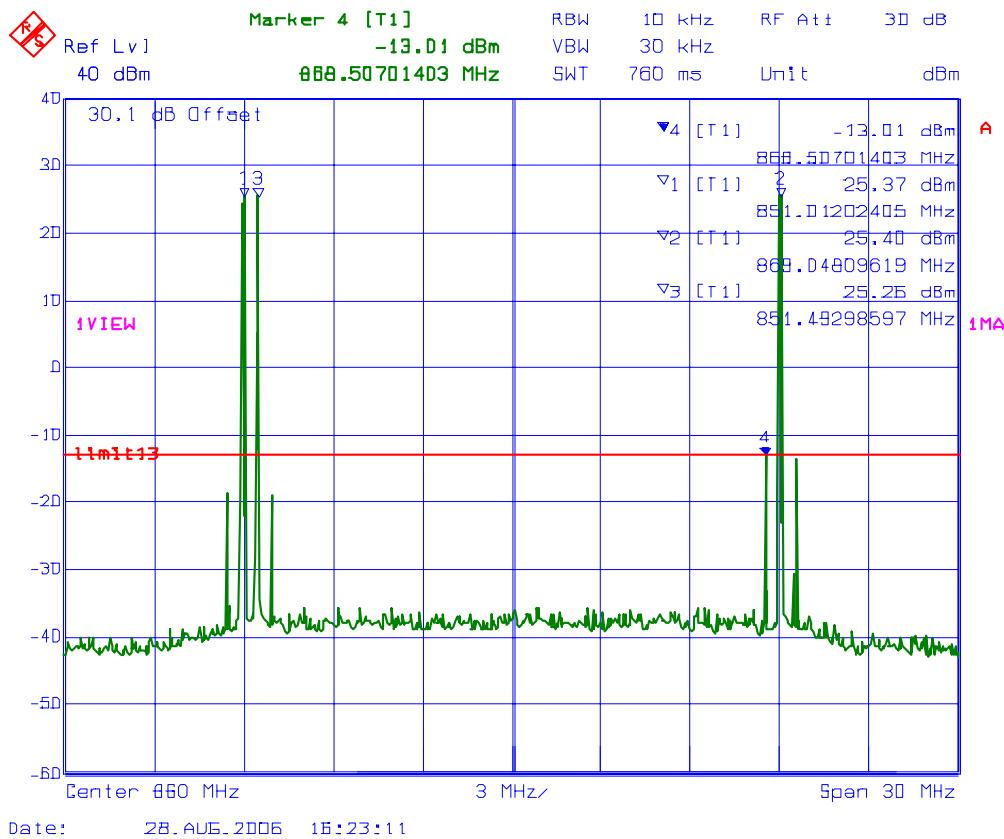
**PLOT #: 12** **Intermodulation with 2 RF signal inputs/outputs**
