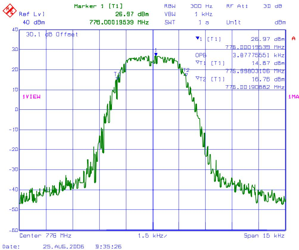
**PLOT # 29 99% Occupied Bandwidth – RF Input Signal**
