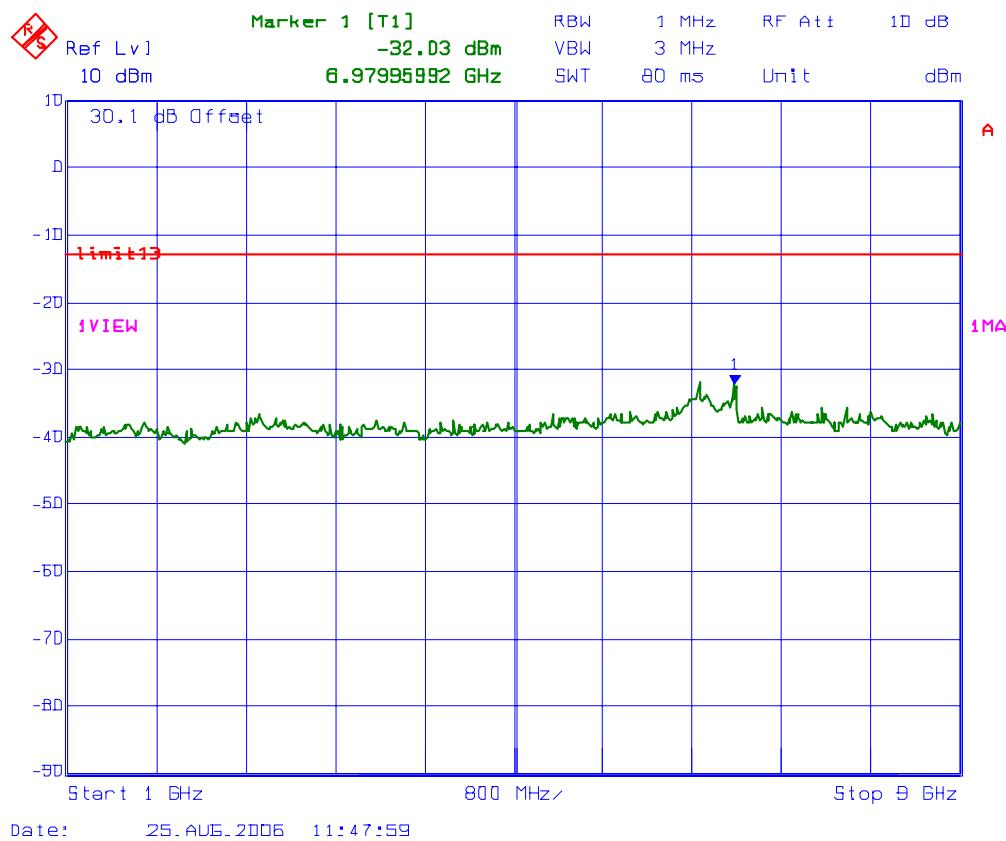
**PLOT # 91    Antenna Conducted RF Spurious Emissions @ Fc: 800 MHz**
