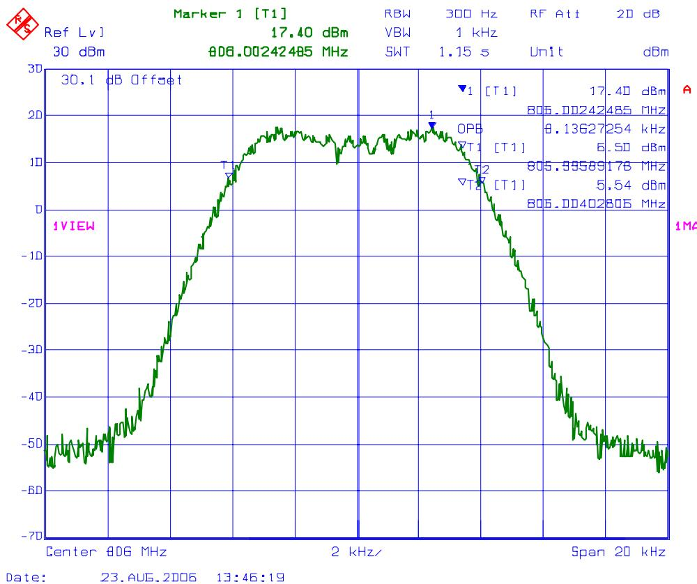
**PLOT # 51 99% Occupied Bandwidth – RF Input Signal**
