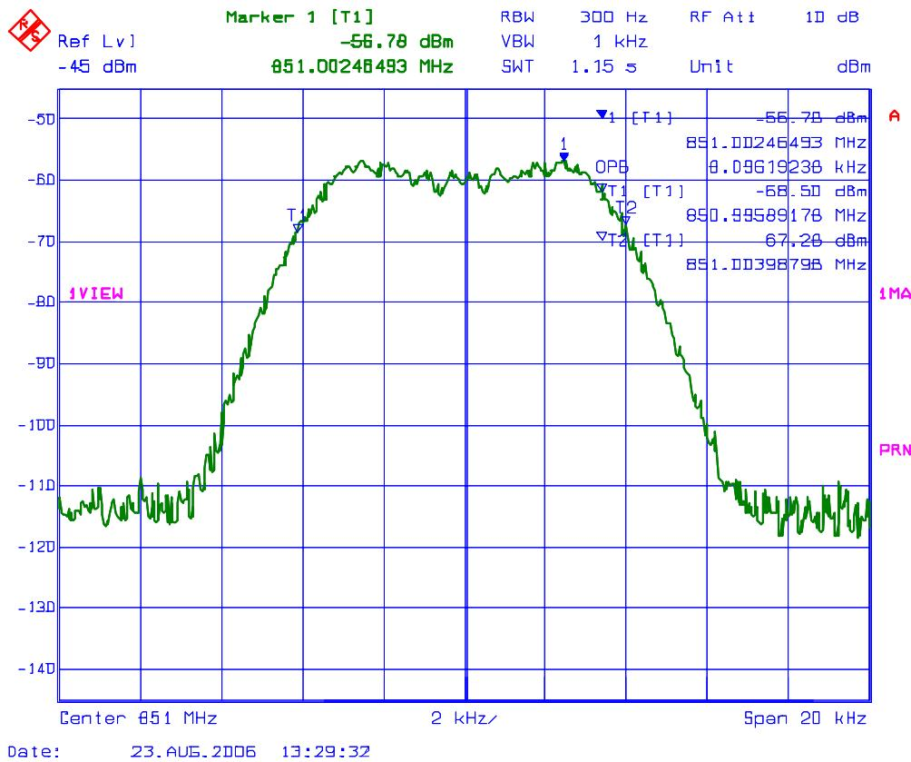
**PLOT # 70 99% Occupied Bandwidth – RF Output Signal**
