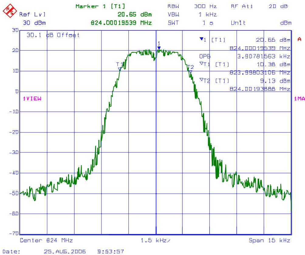
**PLOT # 59 99% Occupied Bandwidth – RF Input Signal**
