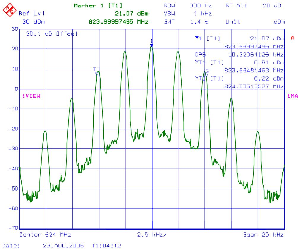
**PLOT # 55 99% Occupied Bandwidth – RF Input Signal**
