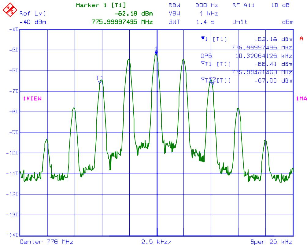
**PLOT # 24 99% Occupied Bandwidth – RF Output Signal**
