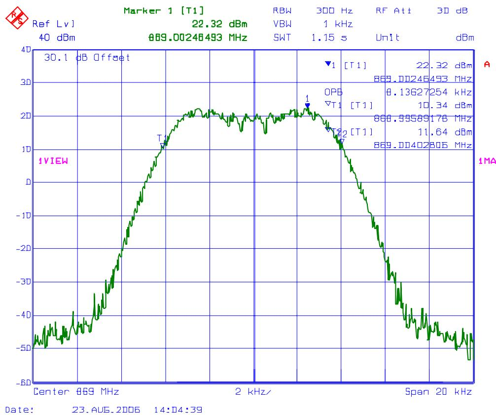
**PLOT # 81 99% Occupied Bandwidth – RF Input Signal**
