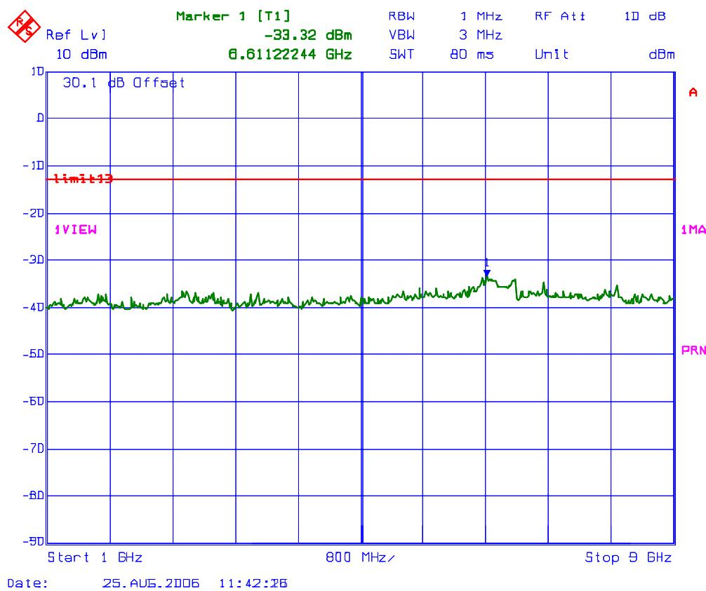
PLOT # 85 Antenna Conducted RF Spurious Emissions @ Fc: 770 MHz
