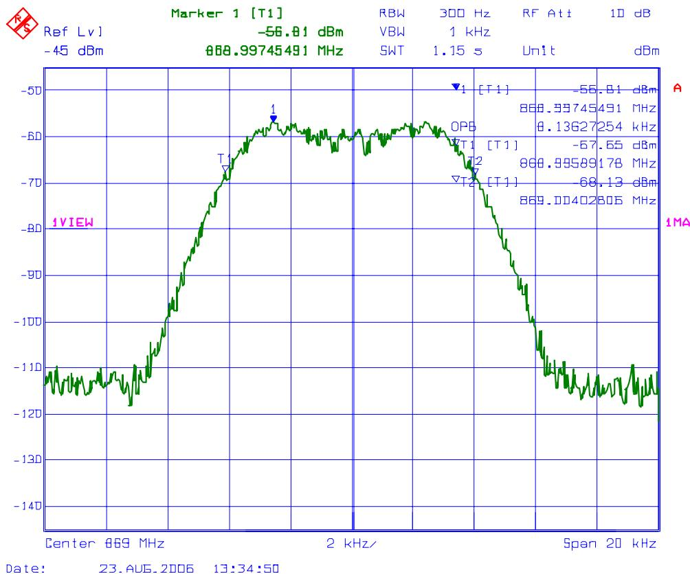
**PLOT # 80 99% Occupied Bandwidth – RF Output Signal**
