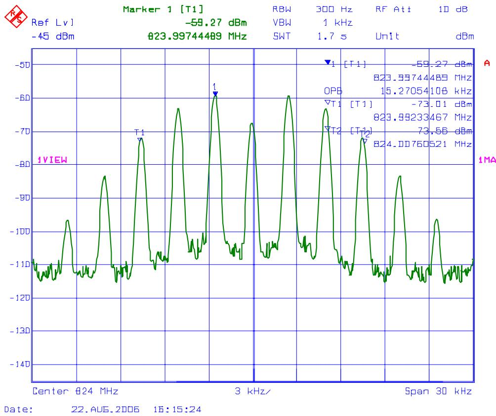
**PLOT # 56 99% Occupied Bandwidth – RF Output Signal**
