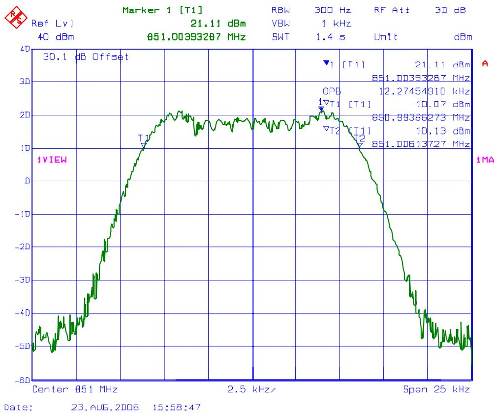
**PLOT # 73 99% Occupied Bandwidth – RF Input Signal**
