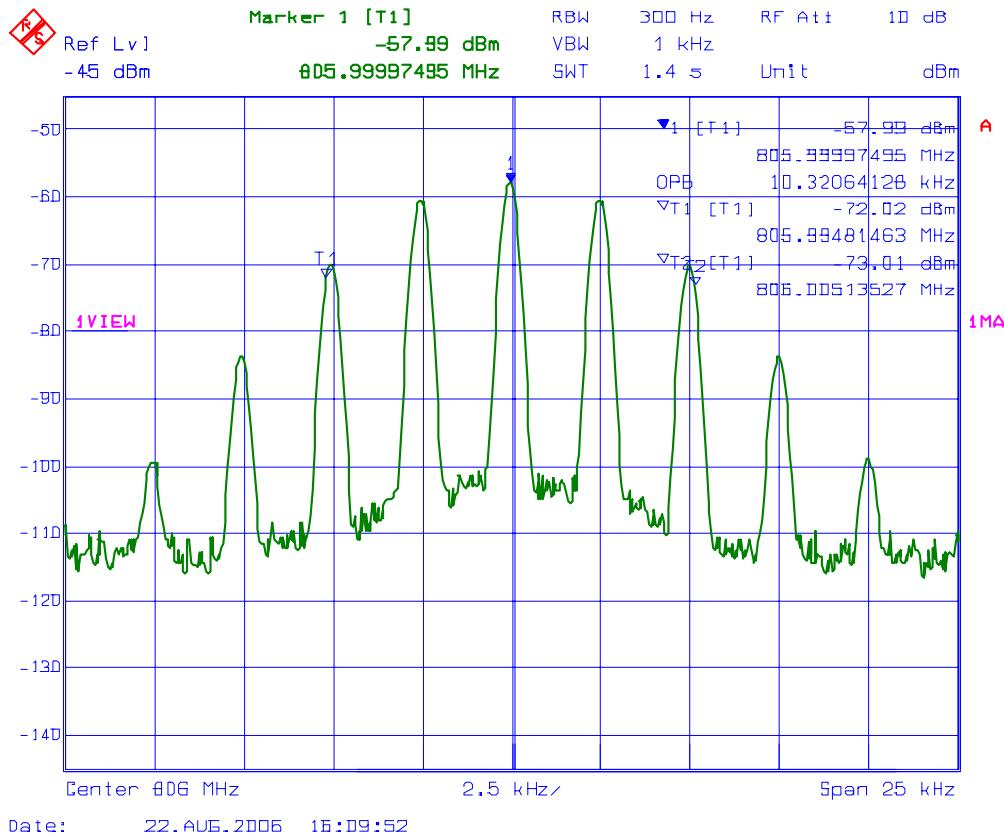
**PLOT # 44** 99% Occupied Bandwidth – RF Output Signal
