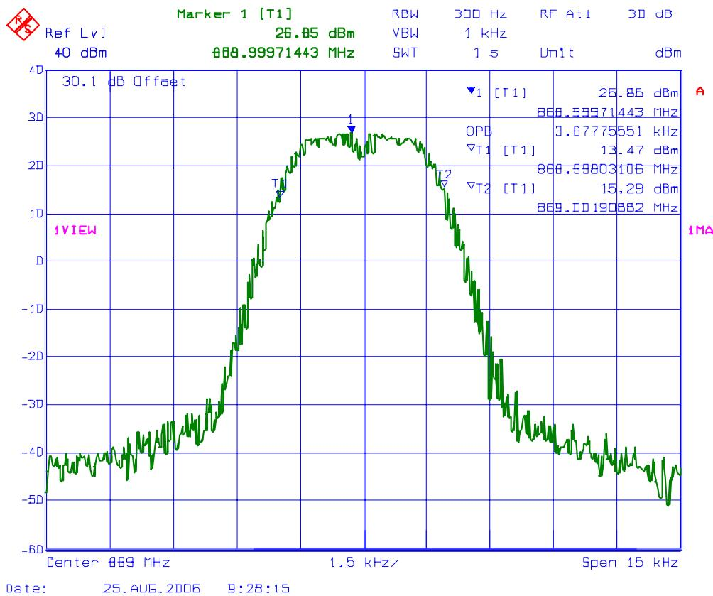
**PLOT # 79 99% Occupied Bandwidth – RF Input Signal**
