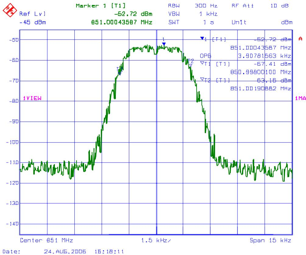
**PLOT # 68 99% Occupied Bandwidth – RF Output Signal**
