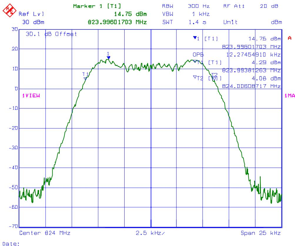
**PLOT # 63 99% Occupied Bandwidth – RF Input Signal**
