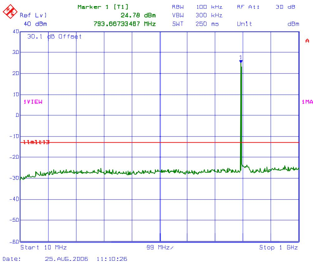
**PLOT # 90    Antenna Conducted RF Spurious Emissions @ Fc: 794 MHz**
