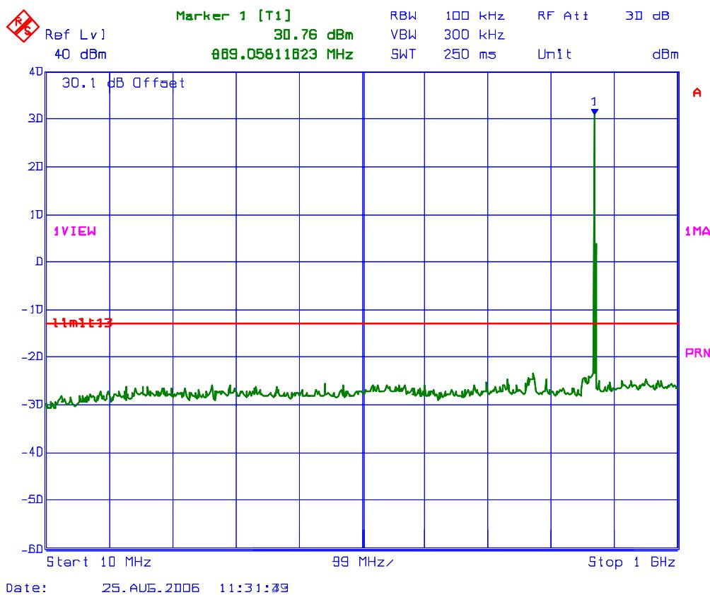
**PLOT # 104 Antenna Conducted RF Spurious Emissions @ Fc: 869 MHz**
