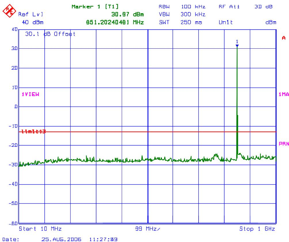
**PLOT # 100 Antenna Conducted RF Spurious Emissions @ Fc: 851 MHz**
