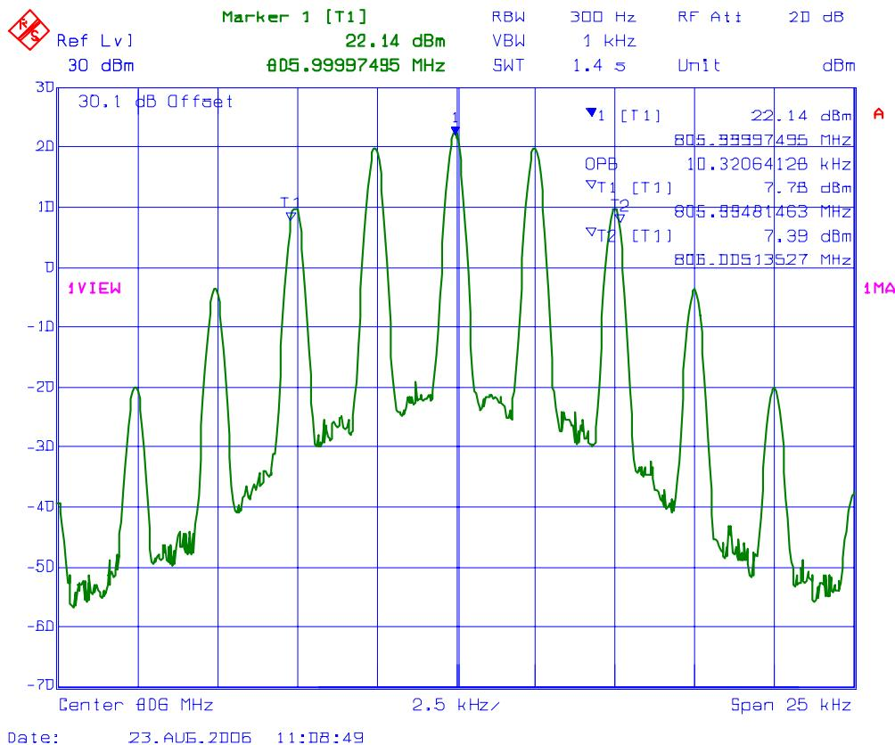
**PLOT # 45 99% Occupied Bandwidth – RF Input Signal**
