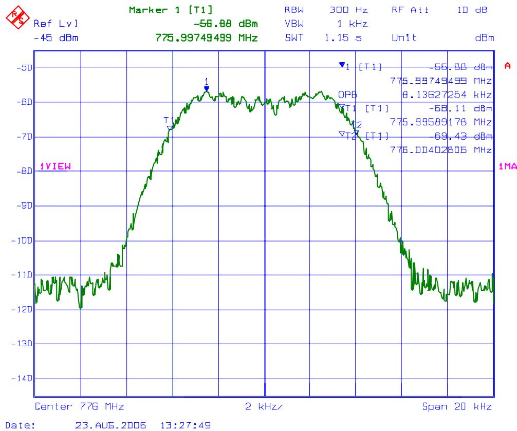
**PLOT # 30 99% Occupied Bandwidth – RF Output Signal**
