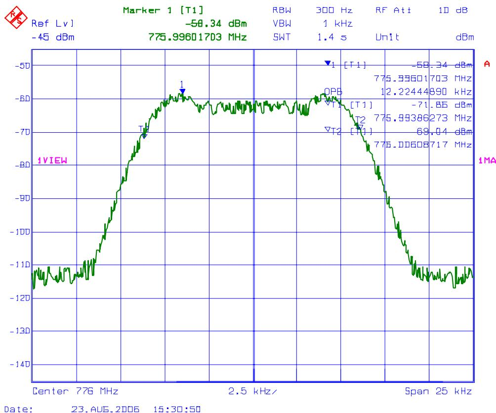
**PLOT # 32 99% Occupied Bandwidth – RF Output Signal**
