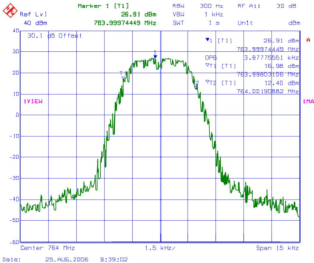
**PLOT # 19 99% Occupied Bandwidth – RF Input Signal**
