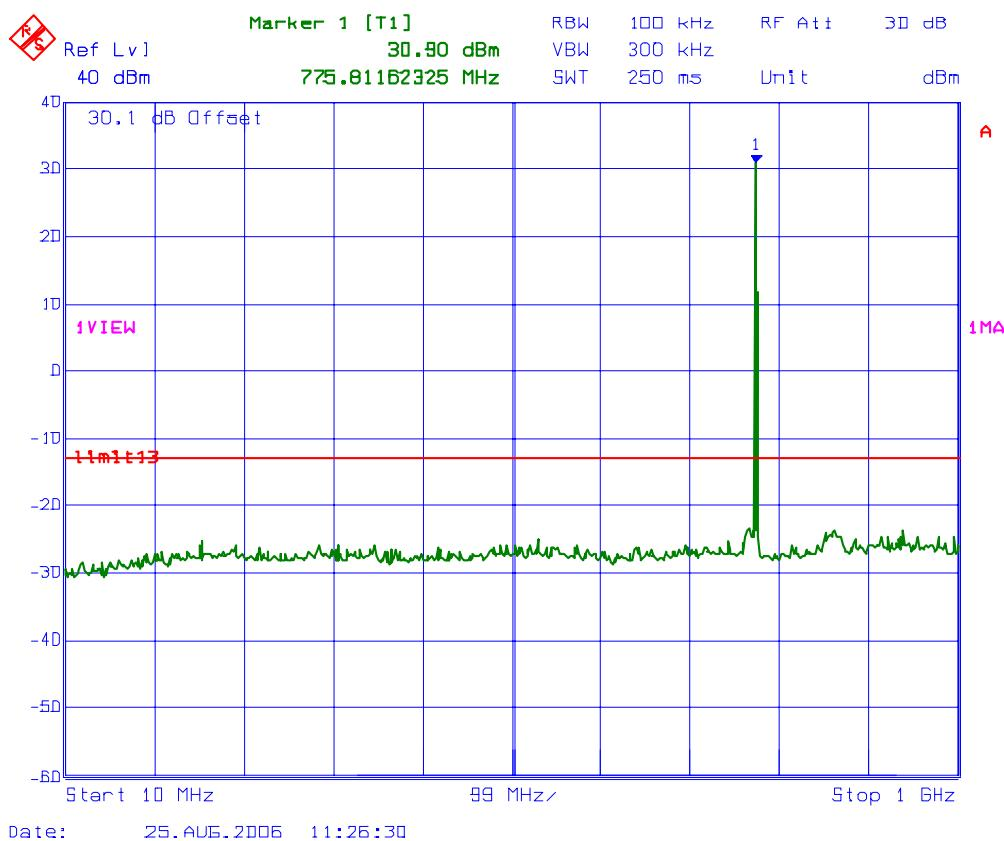
**PLOT # 88    Antenna Conducted RF Spurious Emissions @ Fc: 776 MHz**
