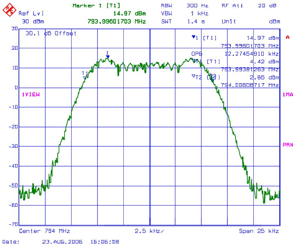
**PLOT # 43 99% Occupied Bandwidth – RF Input Signal**
