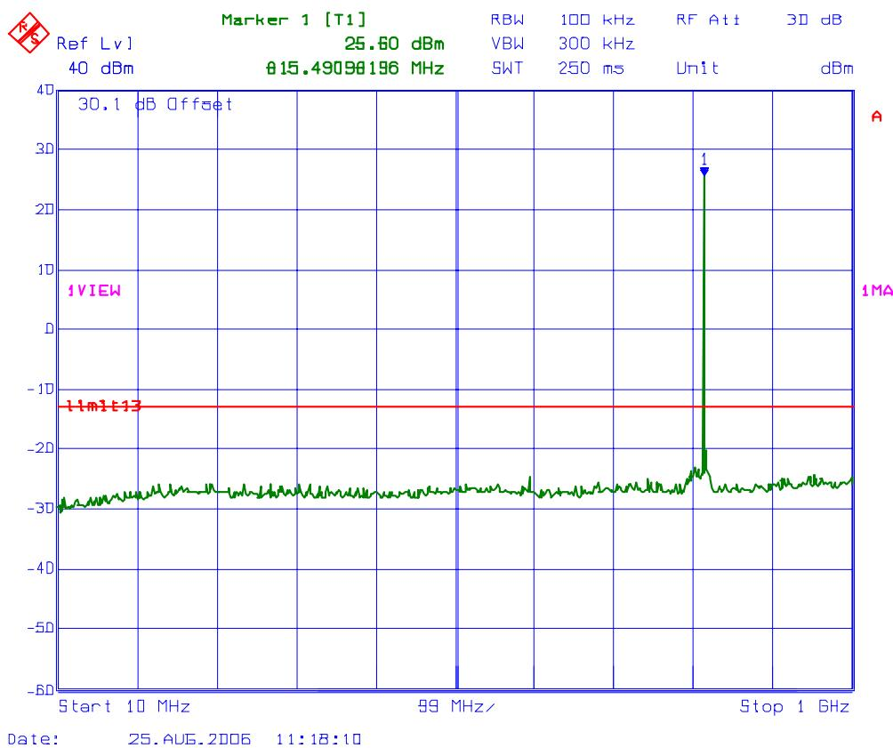
**PLOT # 96    Antenna Conducted RF Spurious Emissions @ Fc: 815 MHz**
