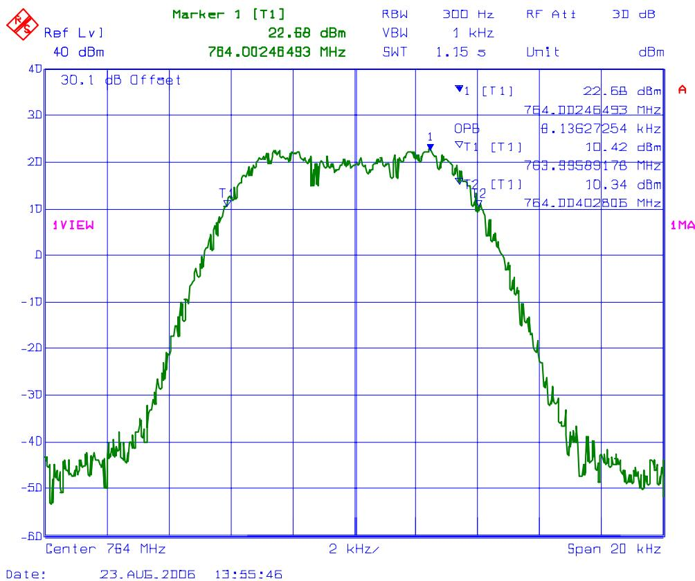
**PLOT # 21 99% Occupied Bandwidth – RF Input Signal**
