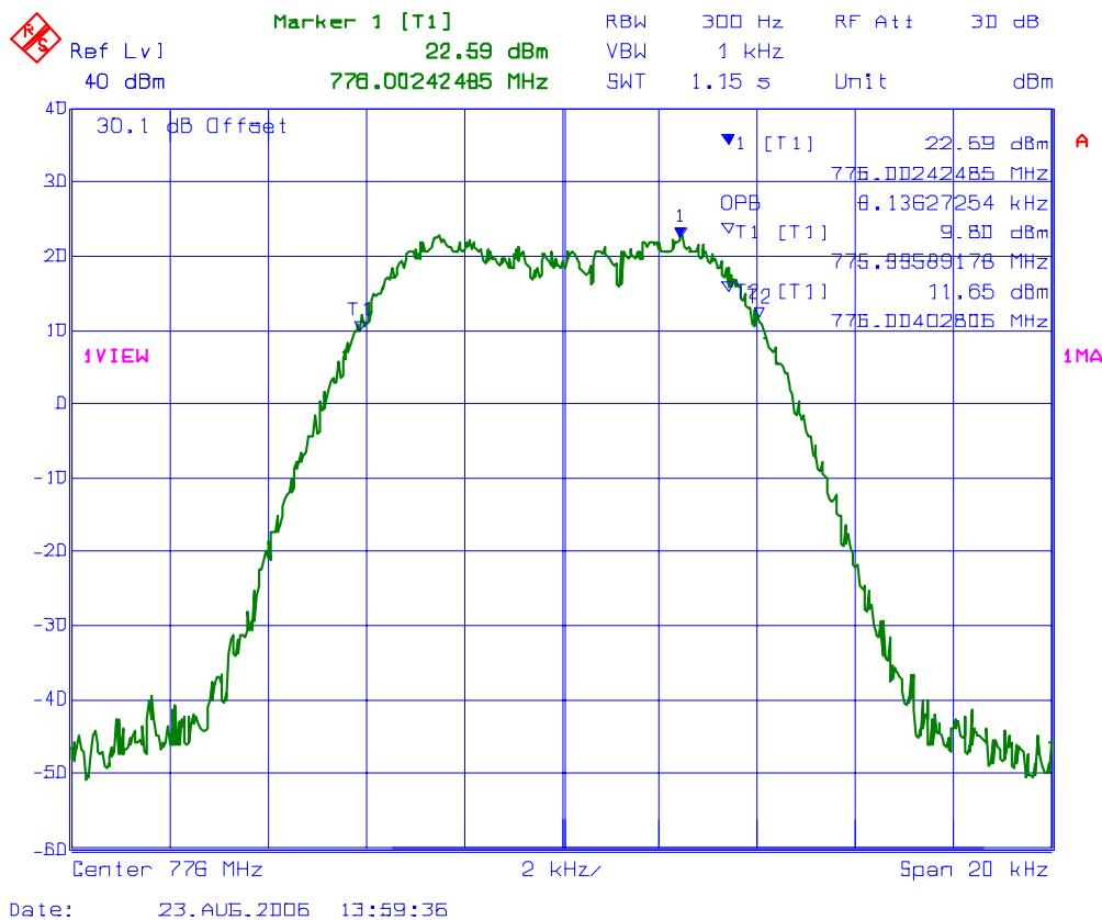
**PLOT # 31 99% Occupied Bandwidth – RF Input Signal**
