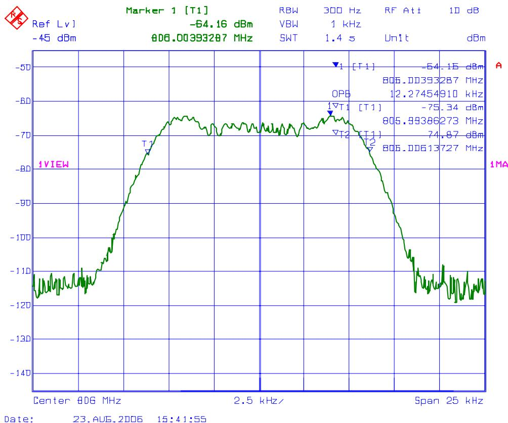
**PLOT # 52 99% Occupied Bandwidth – RF Output Signal**
