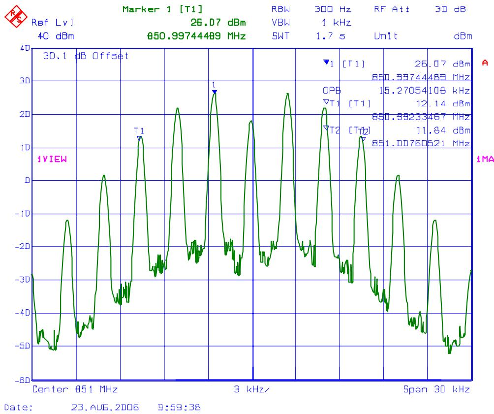
**PLOT # 67 99% Occupied Bandwidth – RF Input Signal**
