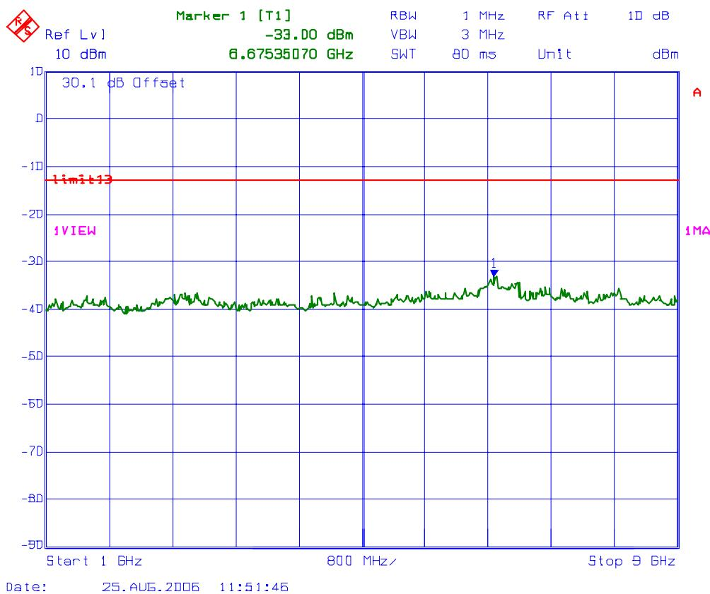
**PLOT # 95 Antenna Conducted RF Spurious Emissions @ Fc: 815 MHz**
