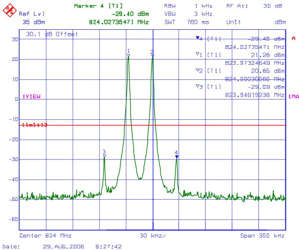
**PLOT #: 10 Intermodulation with 2 RF signal inputs/outputs**
