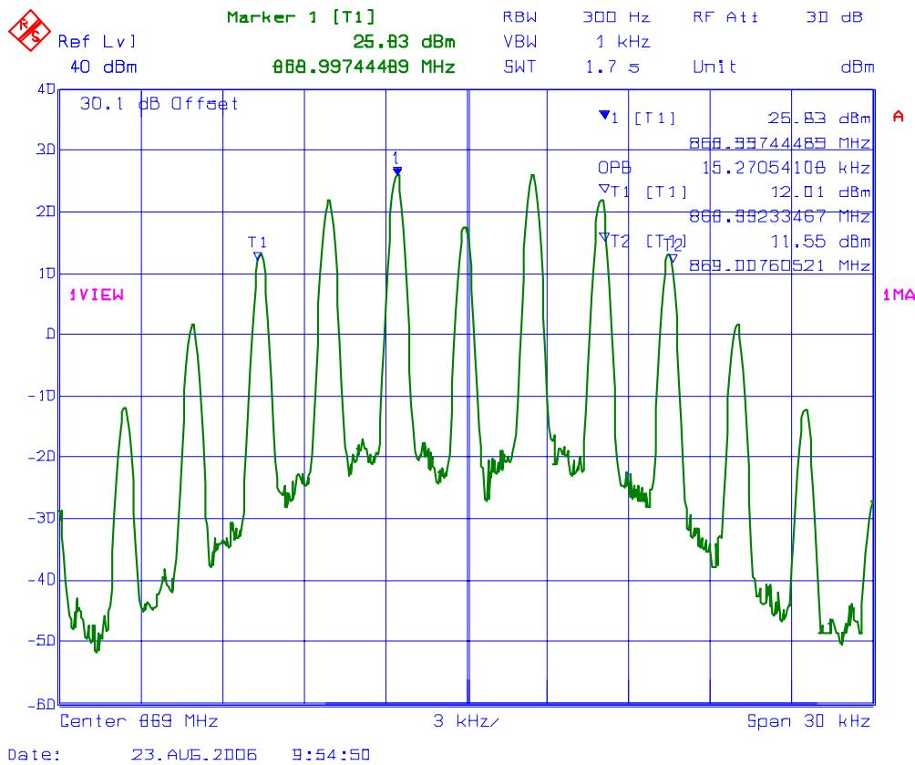
**PLOT # 77 99% Occupied Bandwidth – RF Input Signal**
