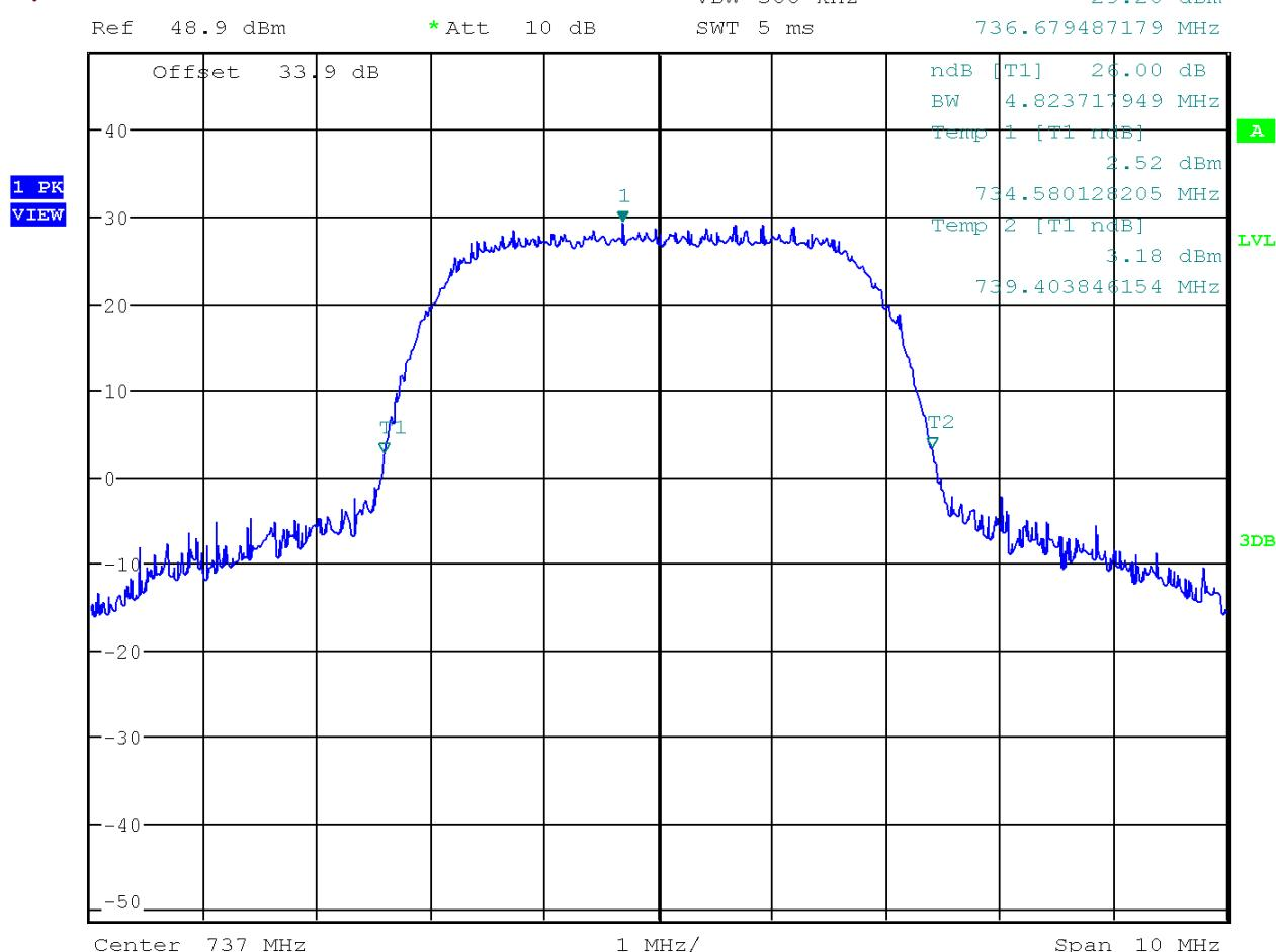
**Input-versus-output spectrum – Downlink with AGC**
