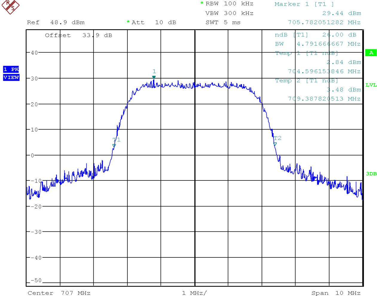
**Input-versus-output spectrum – Downlink without AGC**
