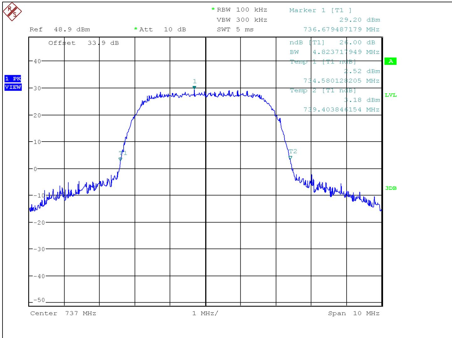
**Input-versus-output spectrum – Downlink with AGC**
