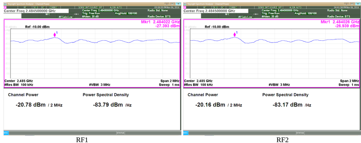
Plot 3.6.8 Band-Edge test results, BW = 8.4 MHz, Data rate = 8 Mbps, Fc = 2475 MHz
