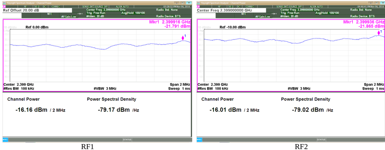
Plot 3.6.8 Band-Edge test results, BW = 8.4 MHz, Data rate = 8 Mbps, Fc = 2475 MHz
