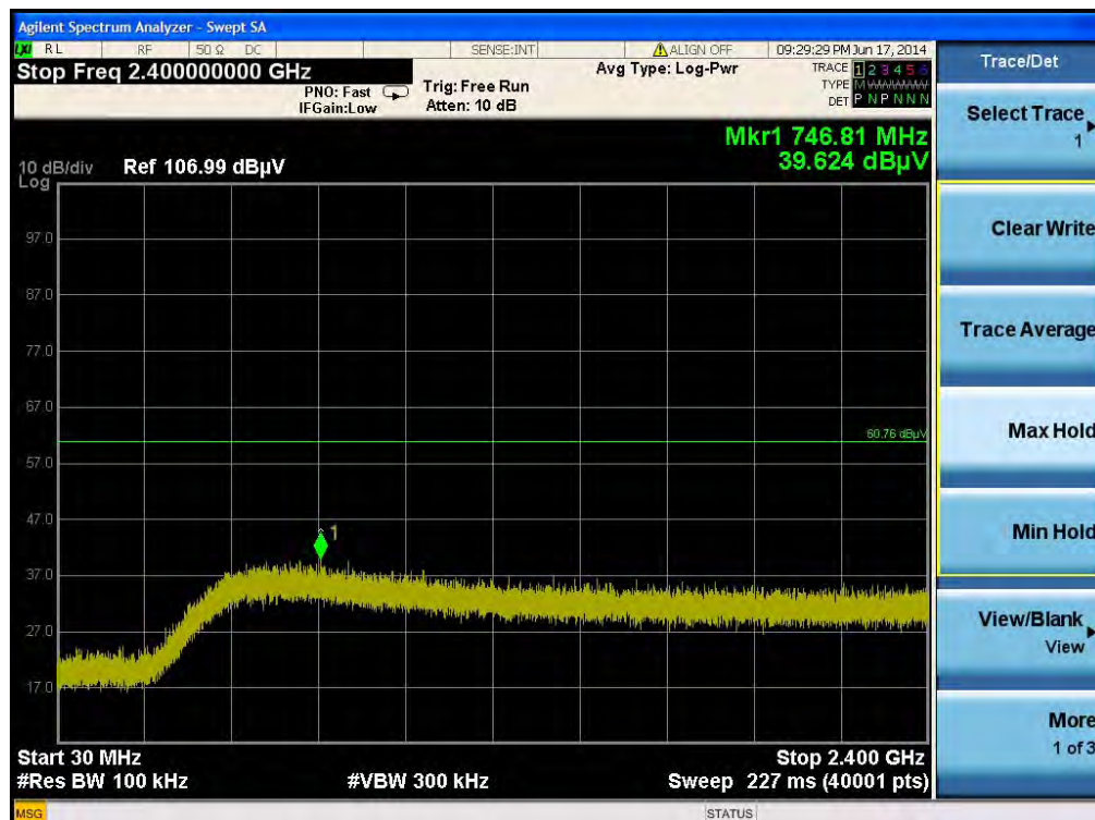
Plot on Configuration IEEE 802.11n MCS0 HT40 / CH 9 / 30MHz~2400MHz (down 30dBc)
