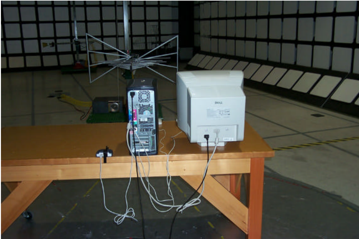
Figure 1 - Radiated Emissions Test Setup
