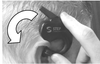
*Gently place the body of the earpiece behind your ear using a slight rotational motion as shown in the diagram.*
