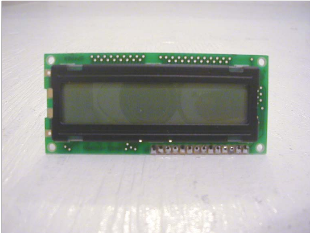
Figure 9: EUT Display module, front view
