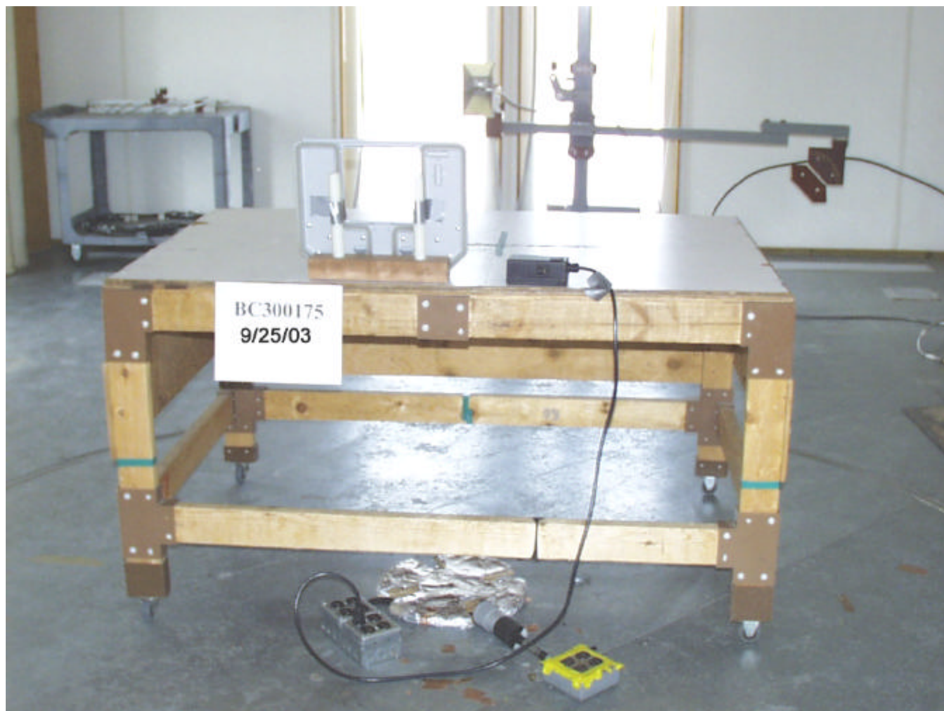
Test-setup photo(s): Radiated Emissions
