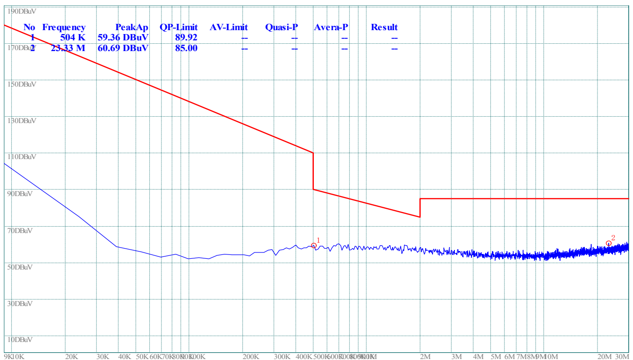
(Plot C.0: 9kHz to 30MHz @ 8-DPSK, channel 78)
