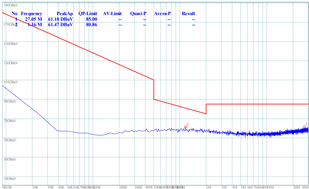
(Plot A.0: 9kHz to 30MHz @ 8-DPSK, channel 0)
