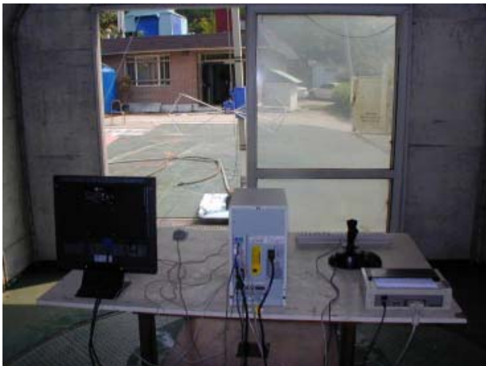
RADIATED EMISSION SETUP PHOTOGRAPH - REAR VIEW ( 30 - 300 MHz )
