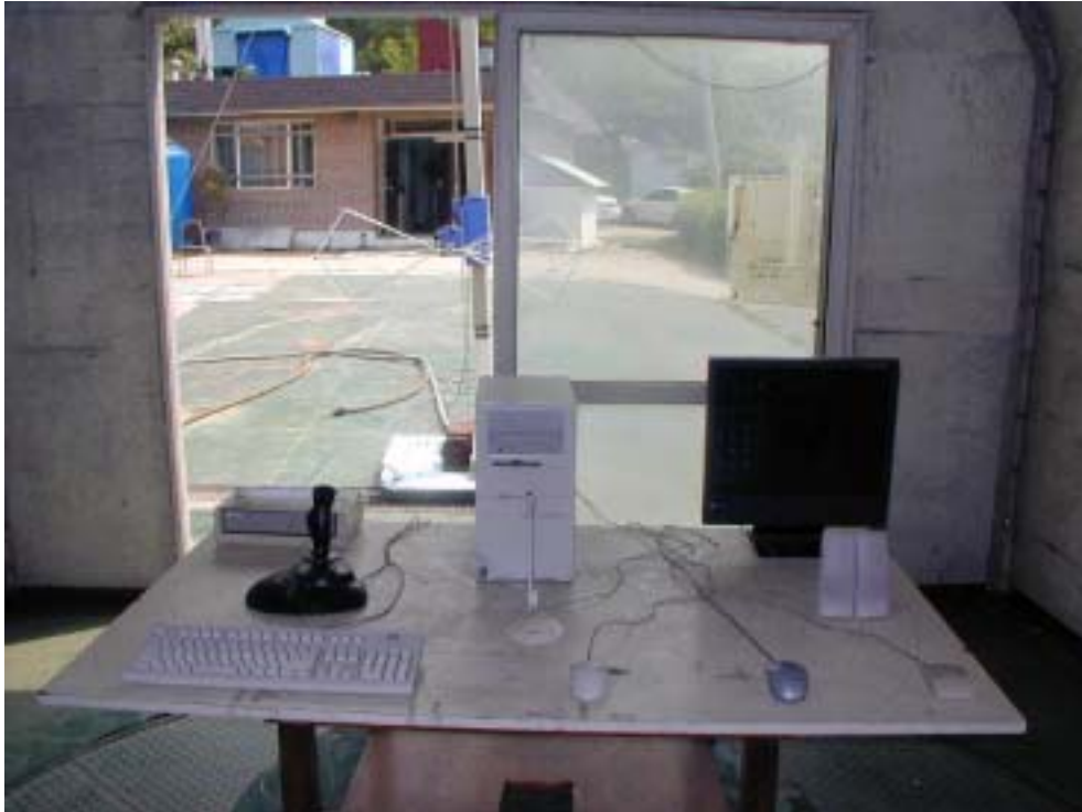
RADIATED EMISSION SETUP PHOTOGRAPH - FRONT VIEW ( 30 - 300 MHz )
