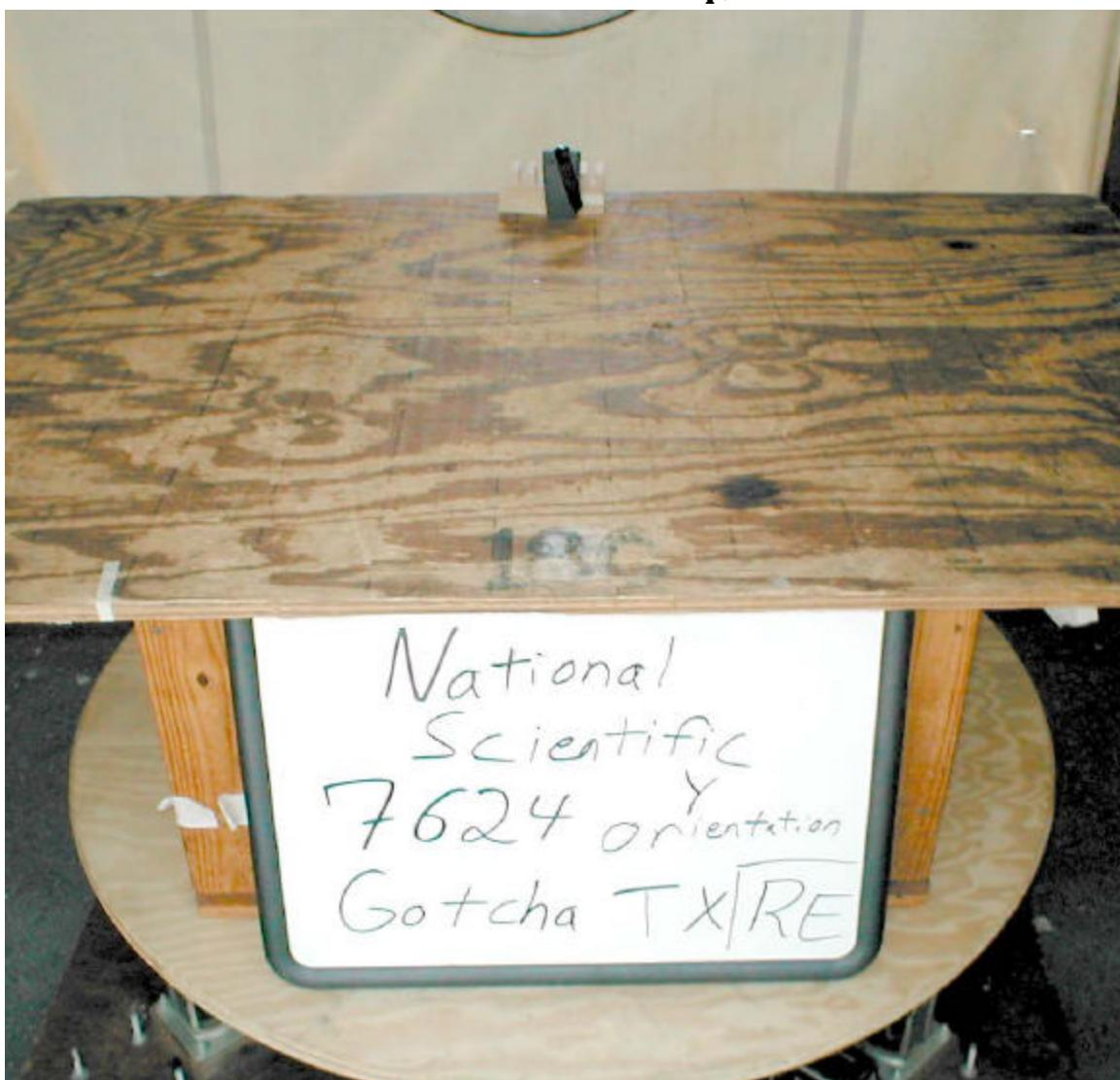
**Radiated Emissions Test Setup, Rear**
